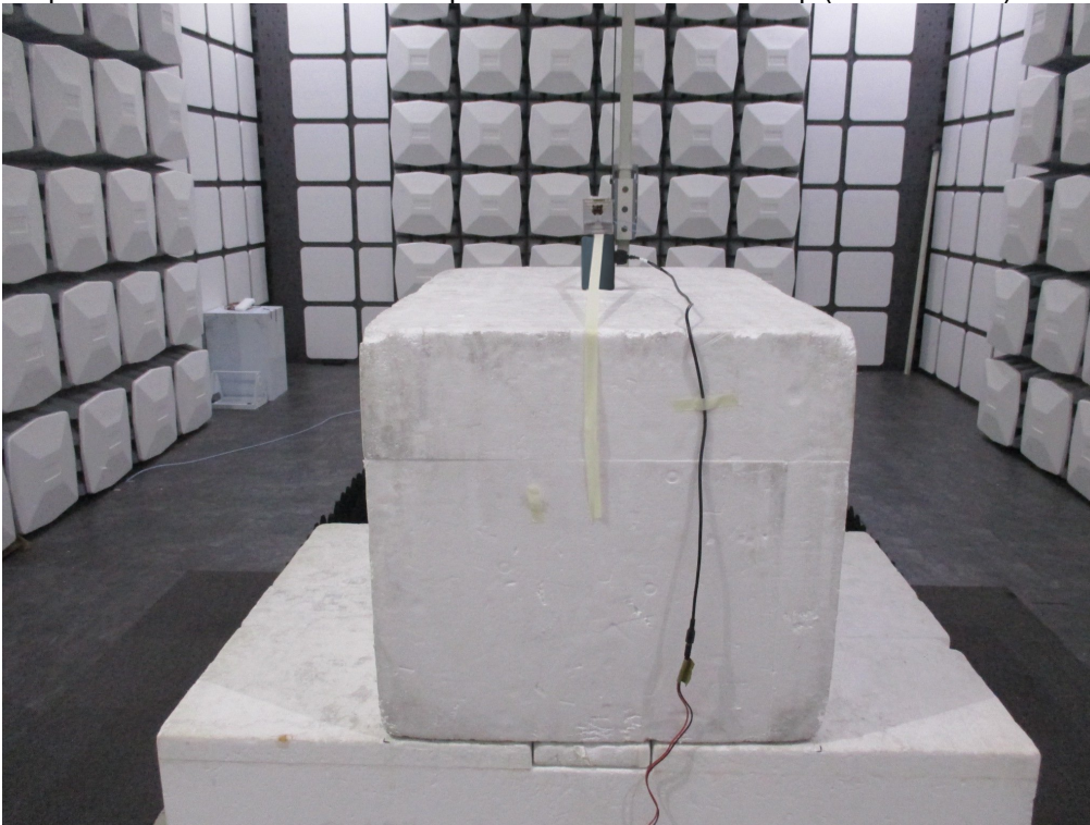
Description: Rear View of Radiated Spurious Emission Test Setup (above 1 GHz)
