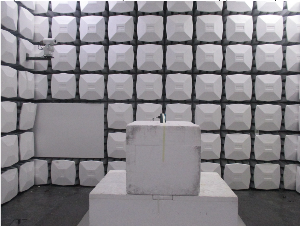
Description: Rear View of Radiated Spurious Emission Test Setup (above 1 GHz)
