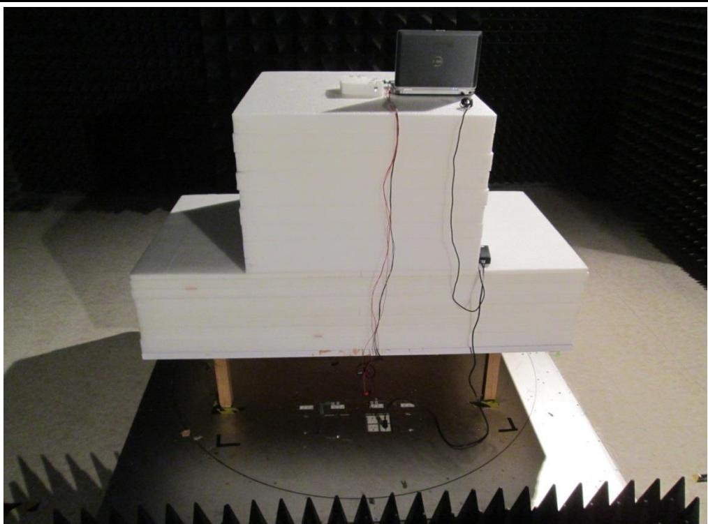
**Radiated Emission Above 1GHz Test**
