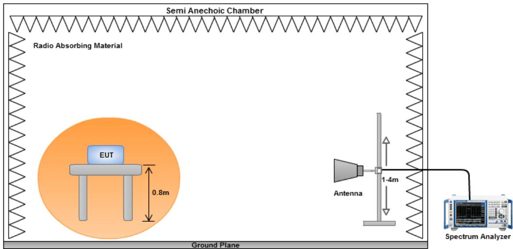
Note: Distance between EUT and antenna is 3 m
