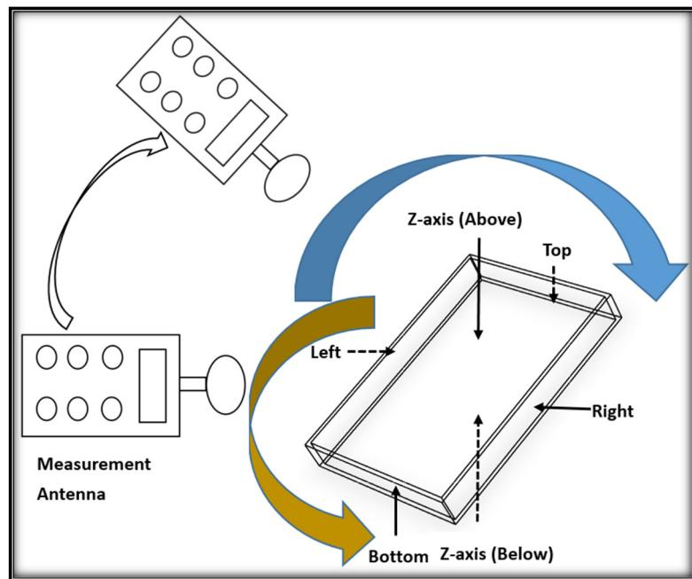
Note: The measurement antenna are moving and surrounding the EUT when performed the test, the test results recorded the highest values for each sides of the EUT (left/right/top/bottom/z-axis (Above)/z-axis (Below))
