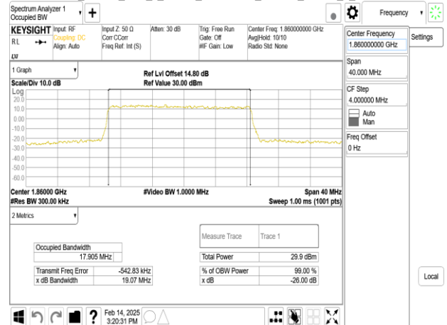
Band2_20MHz_DFT_s_OFDM_SCS15kHz_16QAM_RB100_0_CH376000
