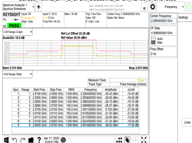
Band38_40MHz_DFT_s_OFDM_SCS30kHz_BPSK_RB1_0_CH518000
