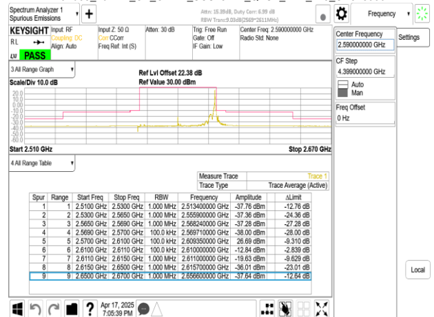
Band38_40MHz_CP_OFDM_SCS15kHz_QPSK_RB216_0_CH518000
