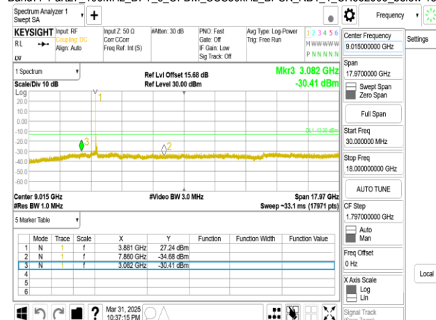
Band77-Part27 100MHz DFT s OFDM SCS30kHz BPSK RB1 1 CH662000 below 18G
