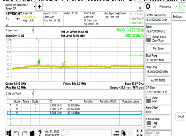
Band77-Part27 100MHz DFT s OFDM SCS30kHz BPSK RB1 1 CH650000 below 18G
