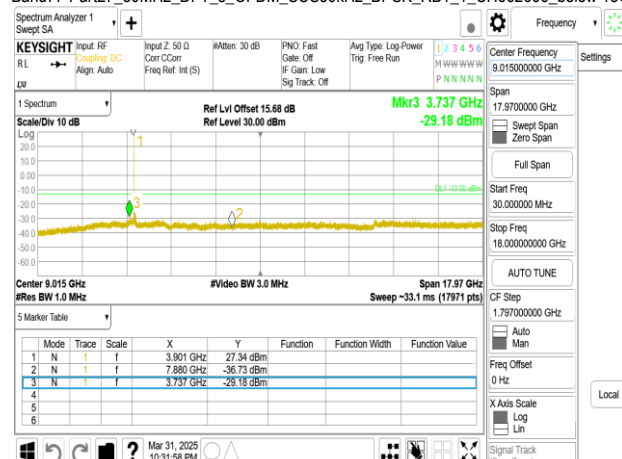
Band77-Part27 80MHz DFT s OFDM SCS30kHz BPSK RB1 1 CH662666 below 18G
