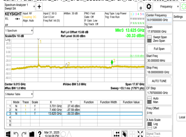
Band77-Part27 90MHz DFT s OFDM SCS30kHz BPSK RB1 1 CH656000 below 18G
