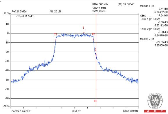
EUT(Client) links with master on 802.11n (HT20) mode
