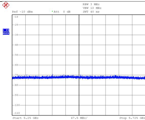
**EUT (Client ) links with master on 802.11n (HT20) mode**
