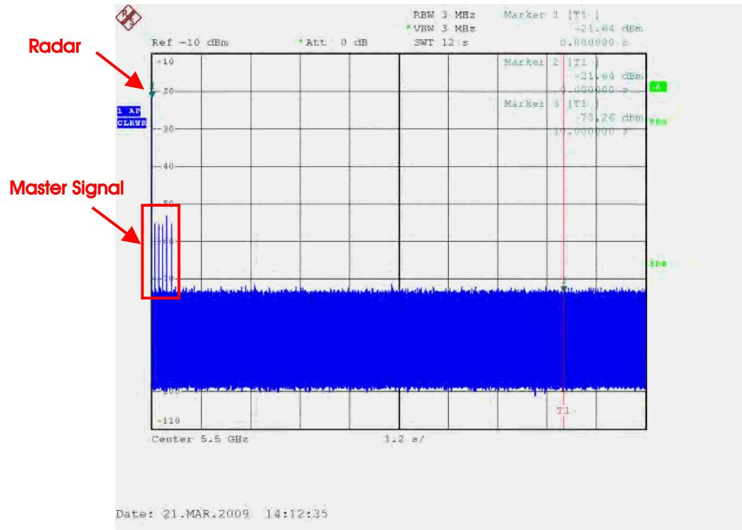
Radar #1 Channel Move Time / 40MHz
