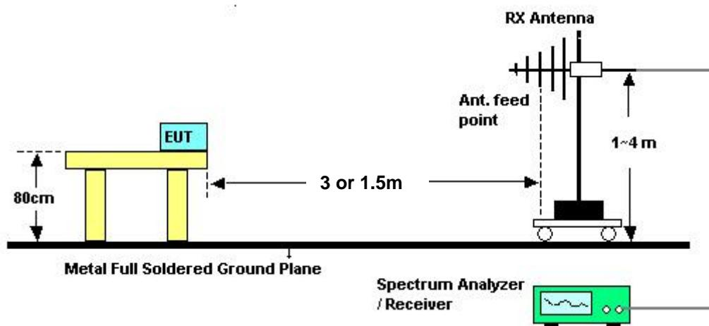
Above 5GHz shall be extrapolated to the specified distance using an extrapolation factor of 20 dB/decade from 3m to 1.5m.
