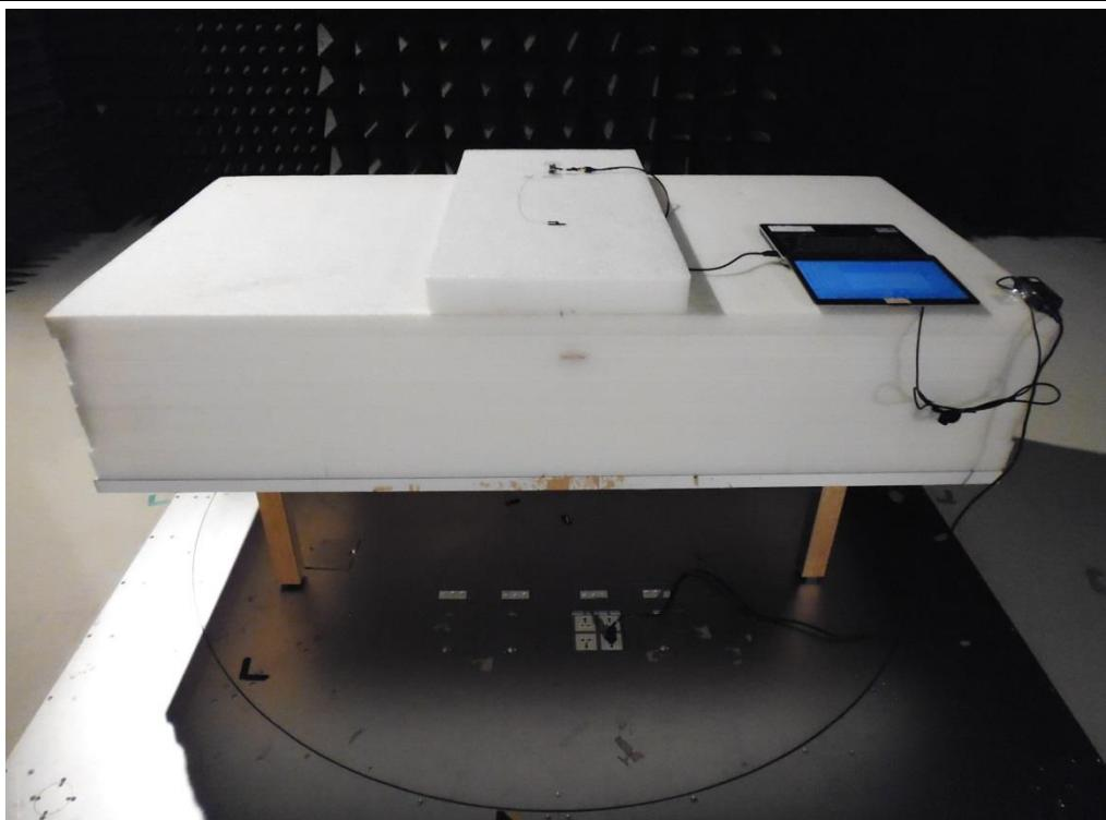
**Radiated Emission Below 1GHz Test**
