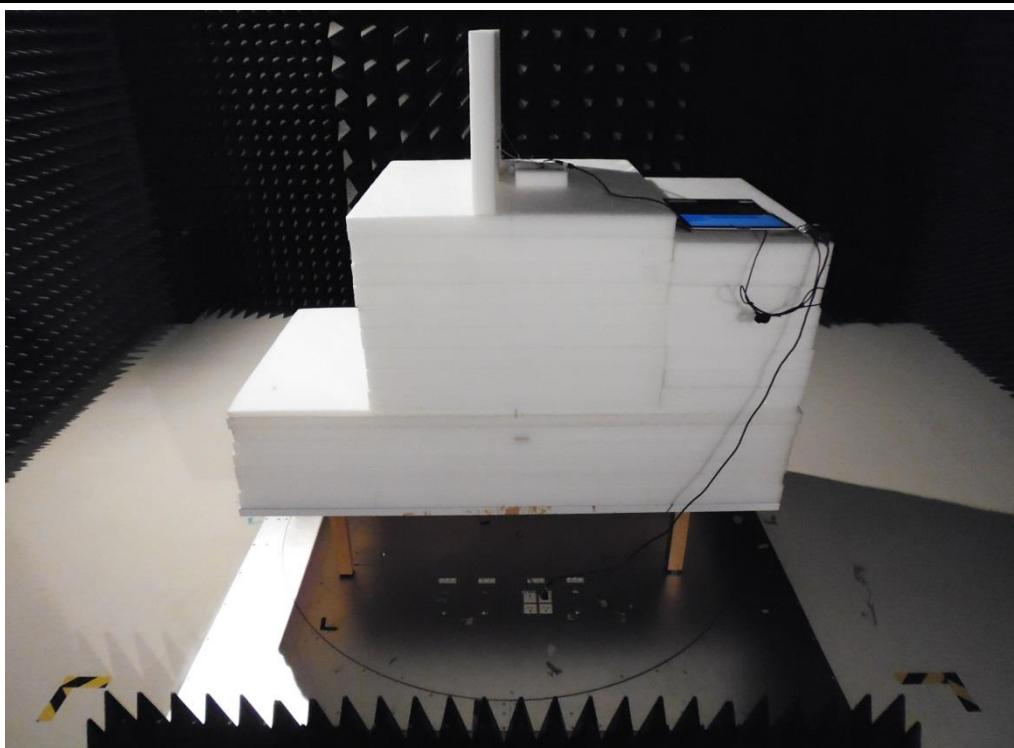
**Radiated Emission Above 1GHz Test**
