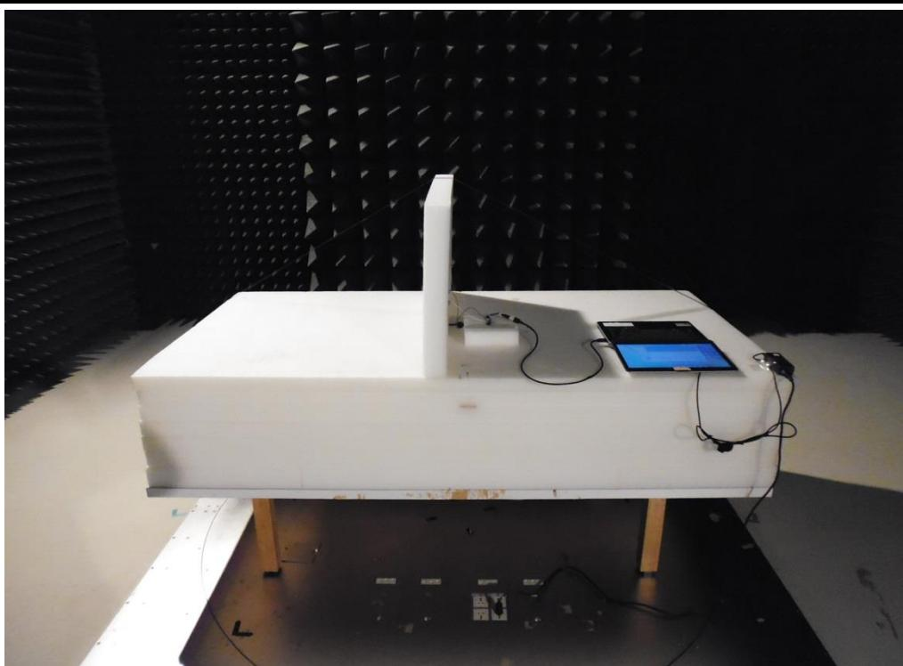
**Radiated Emission Below 1GHz Test**
