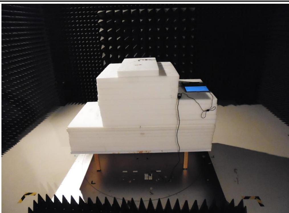
**Radiated Emission Above 1GHz Test**
