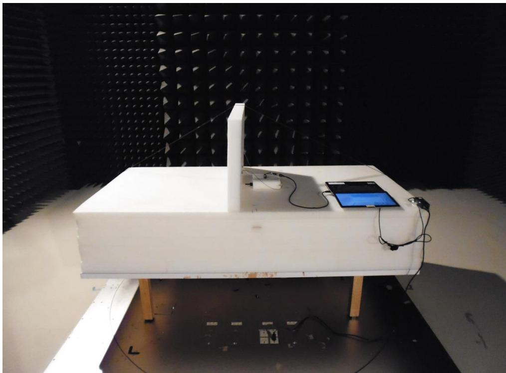
**Radiated Emission Below 1GHz Test**
