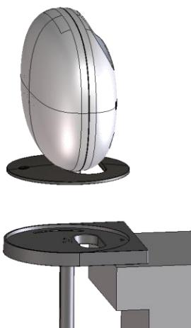
Step 5: Install 2 screws from bottom to prevent rotation (optional)
