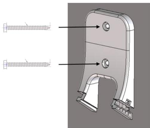
Step 4: Disassemble stand & switch to the device part
