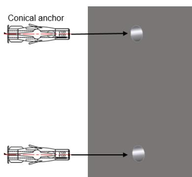
Step 3: Install wall part onto the wall with screw
