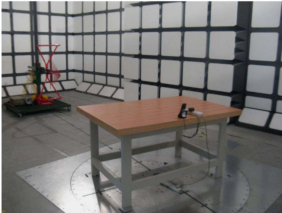
Radiated Emissions - Rear View below 1 GHz for charging mode (model: 31130)
