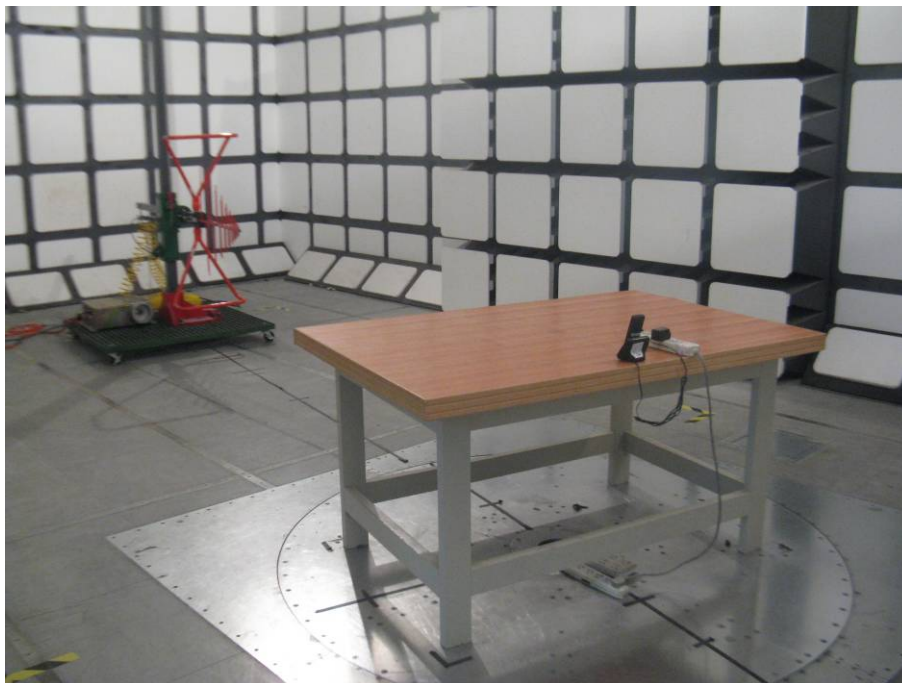
Radiated Emissions - Rear View (30-1000MHz) for charging mode (model 31331)
