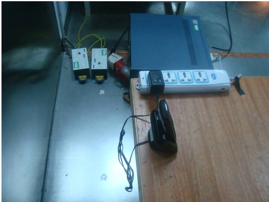
Conducted Emissions - Rear View for charging mode (model 31331)
