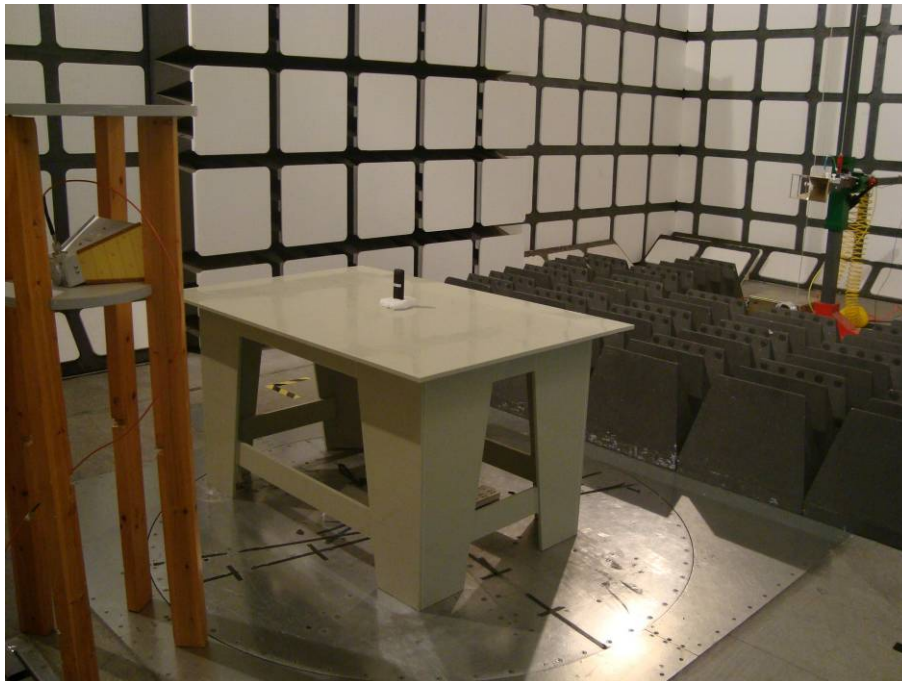
Radiated Emissions - Rear View (Above 1 GHz) for transmitting mode (model: 31331)
