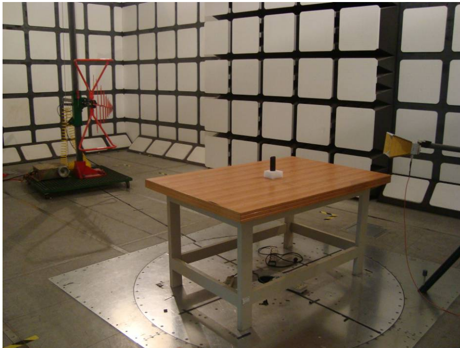
Radiated Emissions - Side View below 1 GHz for transmitting mode (model: 31130)
