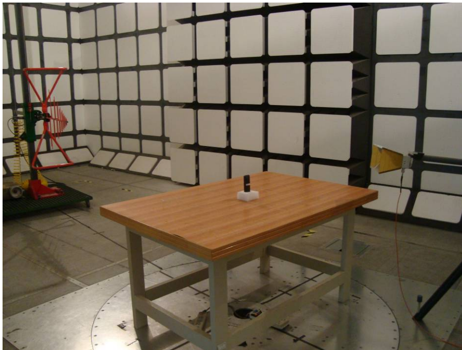
Radiated Emissions - Rear View (30-1000MHz) for transmitting mode (model: 31331)
