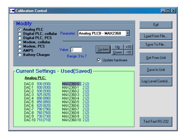
After calibration with power set to maximum increase the span on spectrum Analyzer to 100MHZ, BW Auto and make sure all other signals are at least –45dBc down. Set spectrum Analyzer Span to 100Khz. Exit the calibration window and go back to Ftest window and click on SAT, you should see 5KHZ tone on carrier. Click on ST and you should see 10KHZ tone on carrier. Now we will do calibration on Audio for compressor and expander.
