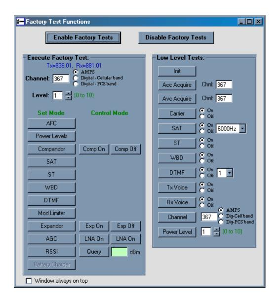
Click on Enable factory test and then click on power levels. Now you should be able to see analog transmit on Spectrum Analyzer. Exit this window and go to calibration table again and select analog plc, for analog mode calibration. Use the power meter and calibrate the output power for first four level at +27.7dBm(600mW) and every other level 4dB less.
