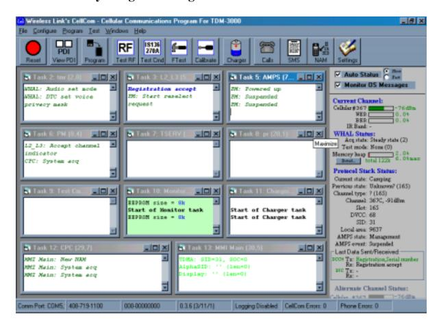
To be able to see every thing, make sure on left hand side of CellCom Auto Status and Monitor are checked on. If you have a green indication for the channel on left hand side of CellCom window, that means your receive side is working. Reduce the RF level on IFR to –105dBm, There should be no more than 3% to 4%BER indication on left hand side of CellCom window. If OK go to step 21. If there are more than 4% we have to check receive path. If the indication is red, this means you are not synch to
