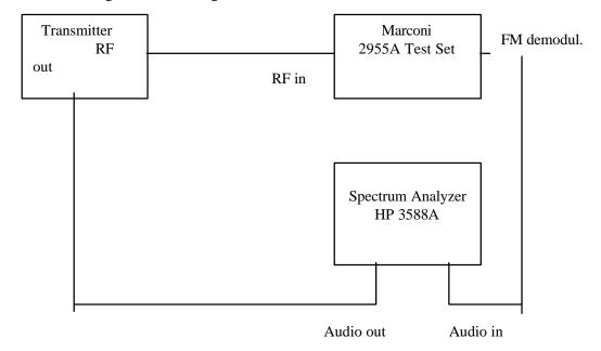
On that block diagram, the HP 3885A spectrum analyzer having the tracing generator, and the Marconi 2955A Radio Communication Test Set having an output of a FM demodulator, are used. After the calibration was made (the -20 dBm reading of the spectrum analyzer corresponds to the 9 kHz deviation) the spectrum analyzer was set to scan the frequency from 300 Hz to 30 kHz, with the same audio input level as described above, and with compressor OFF and expander OFF.
