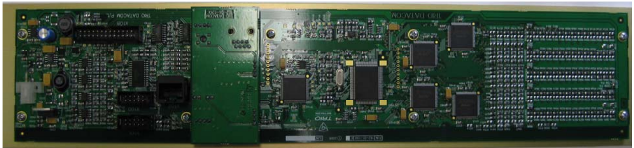
Base station power amplifier shielding removed
