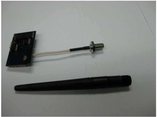
View #2 of Module with SMA Antenna
