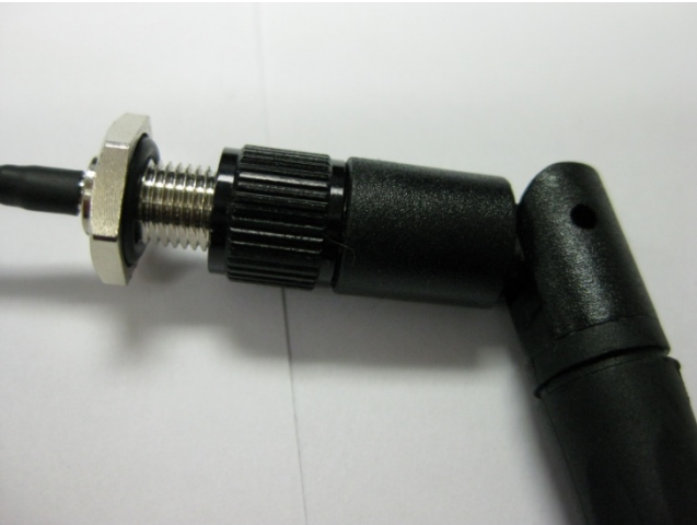
Close Up of SMA Antenna in Bent Position
