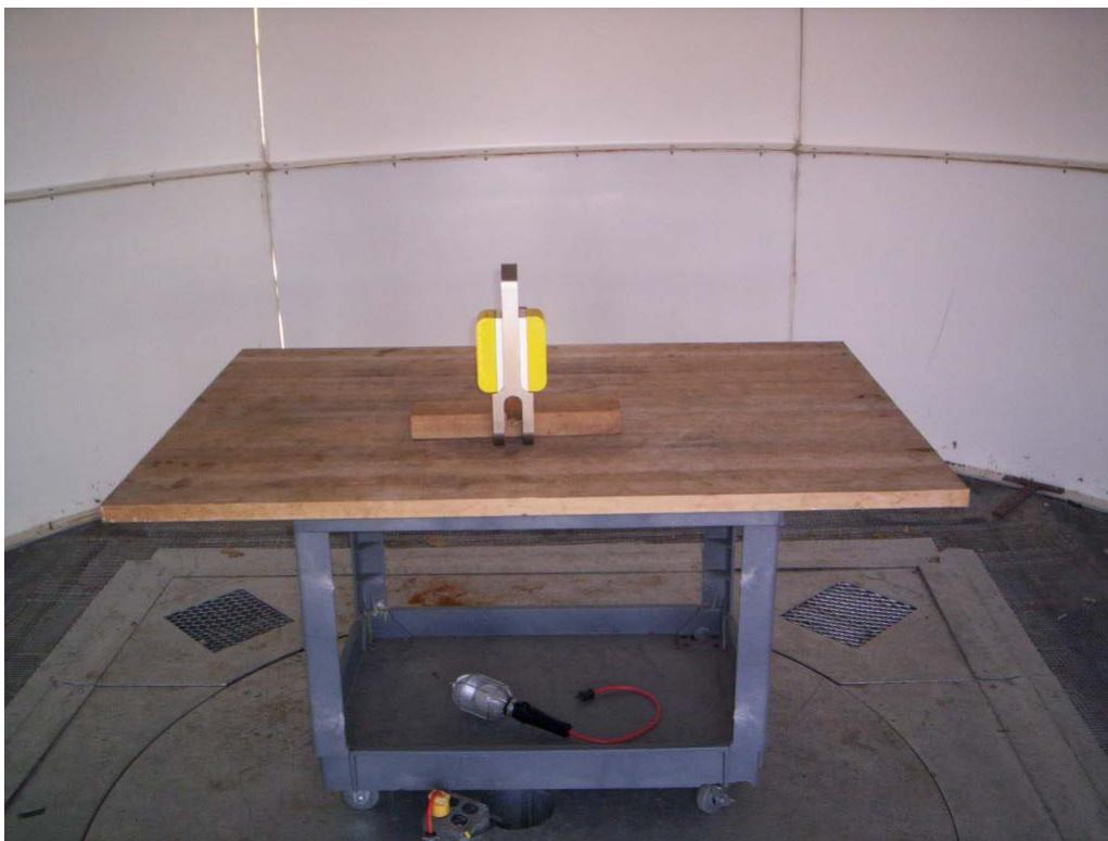
**Appendix C : Block Diagram of Test Setups****Test Site For Radiated Emissions**
