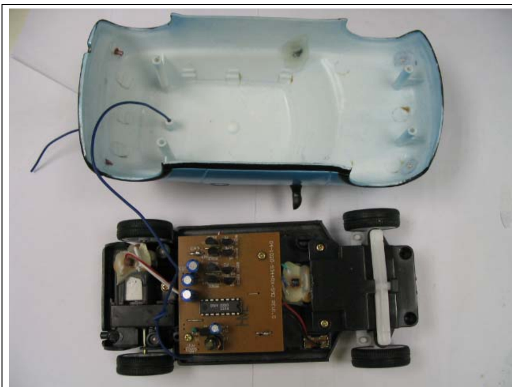
Receiver (Internal view)
