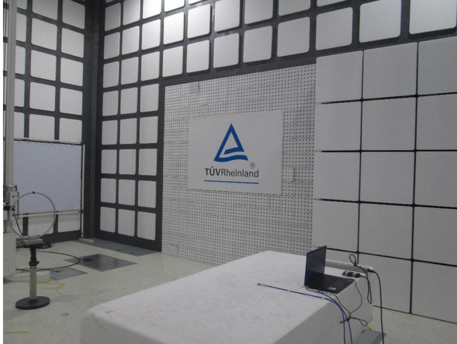
Photograph 3: Test Setup for Spurious Emissions (Back View 1)
