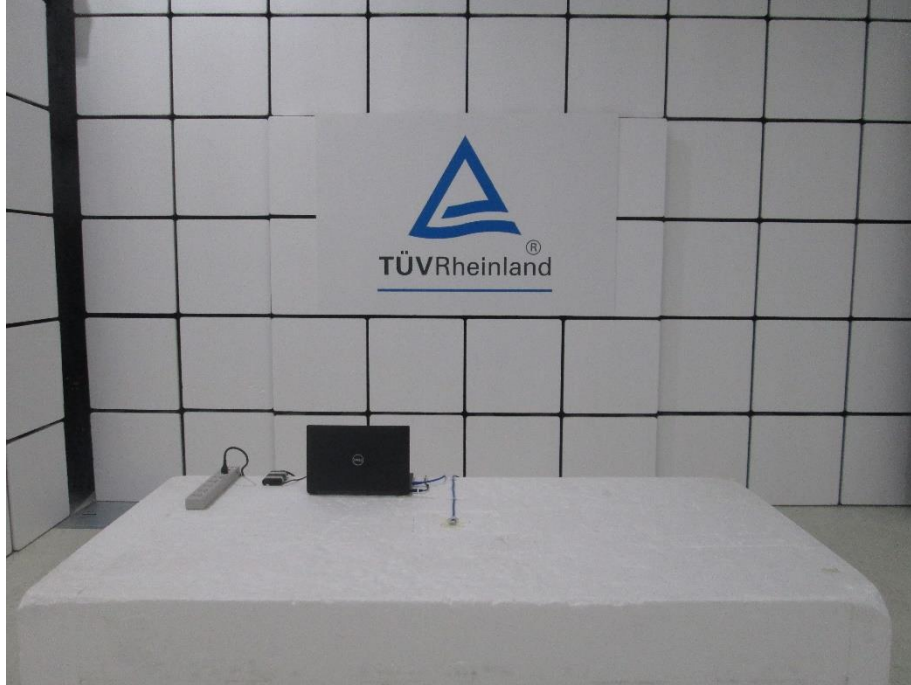
Photograph 1: Test Setup for Spurious Emissions (Front View 1)
