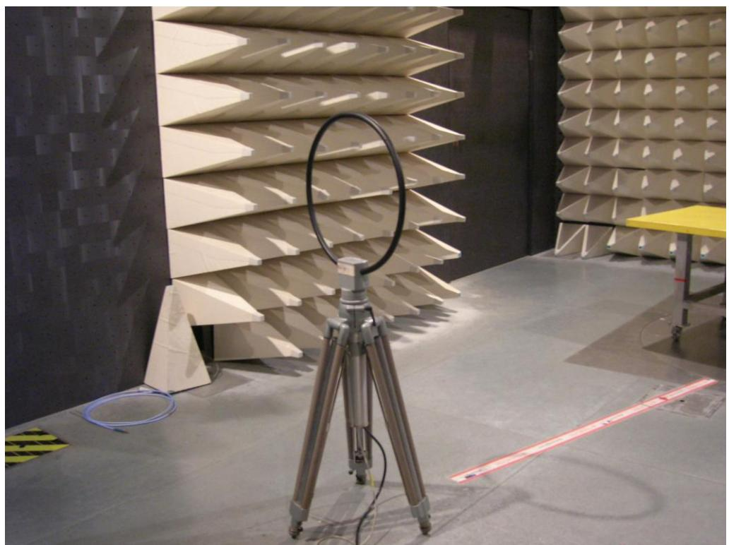
For radiated emissions 30MHz~1GHz
