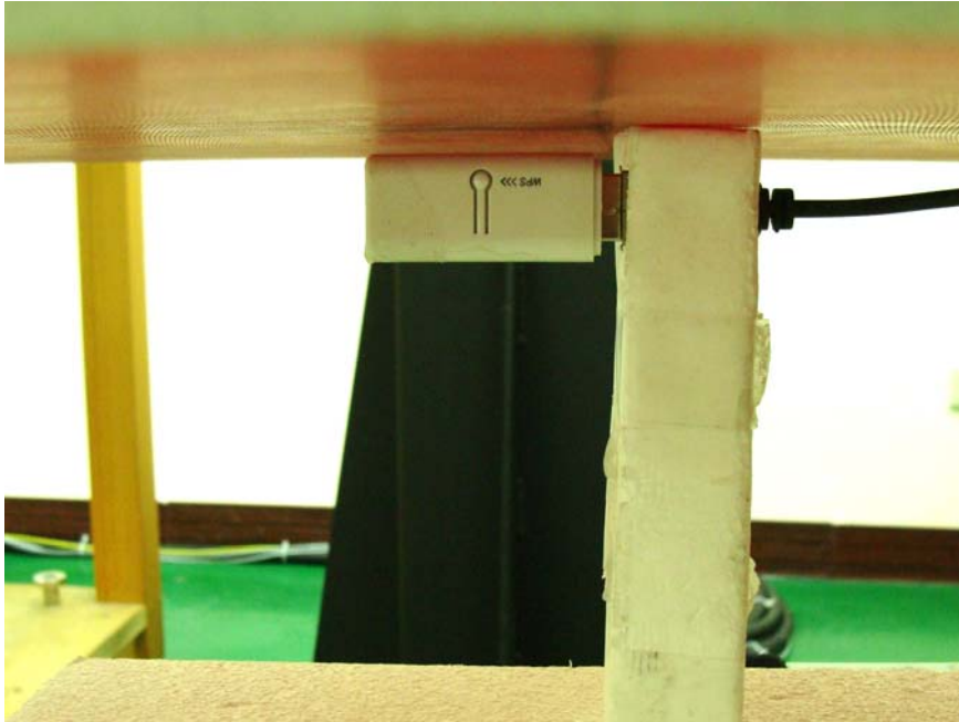
USB Configuration 3 with Phantom 5 mm Gap (Vertical Front)
