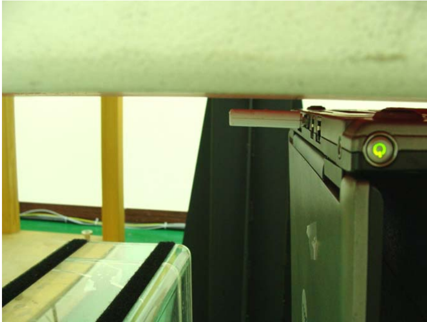
USB Configuration 1 with Phantom 10 mm Gap for Back-off SAR (Horizontal Up)
