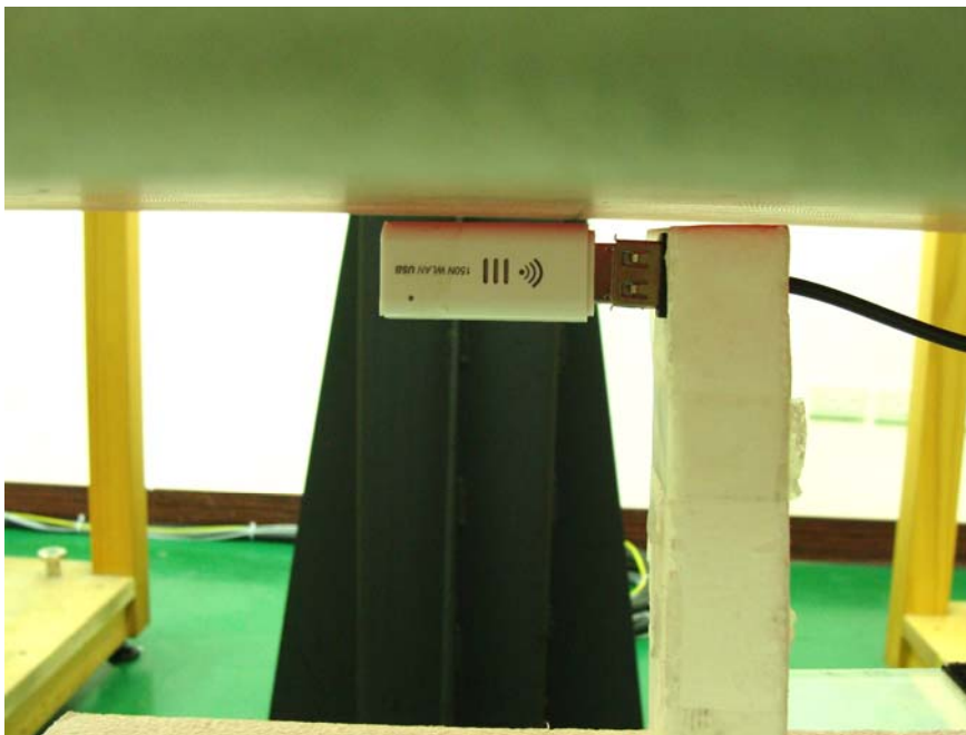
USB Configuration 4 with Phantom 5 mm Gap (Vertical Back)
