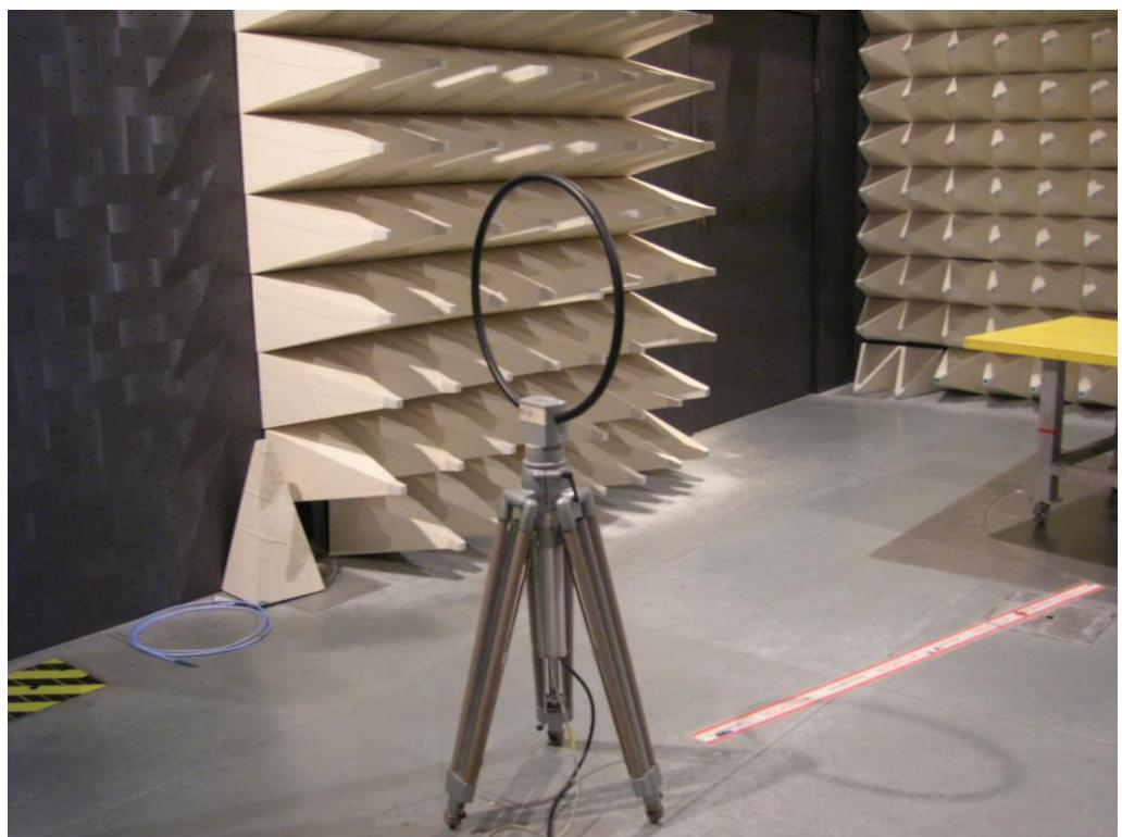
For radiated emissions 30MHz~1GHz
