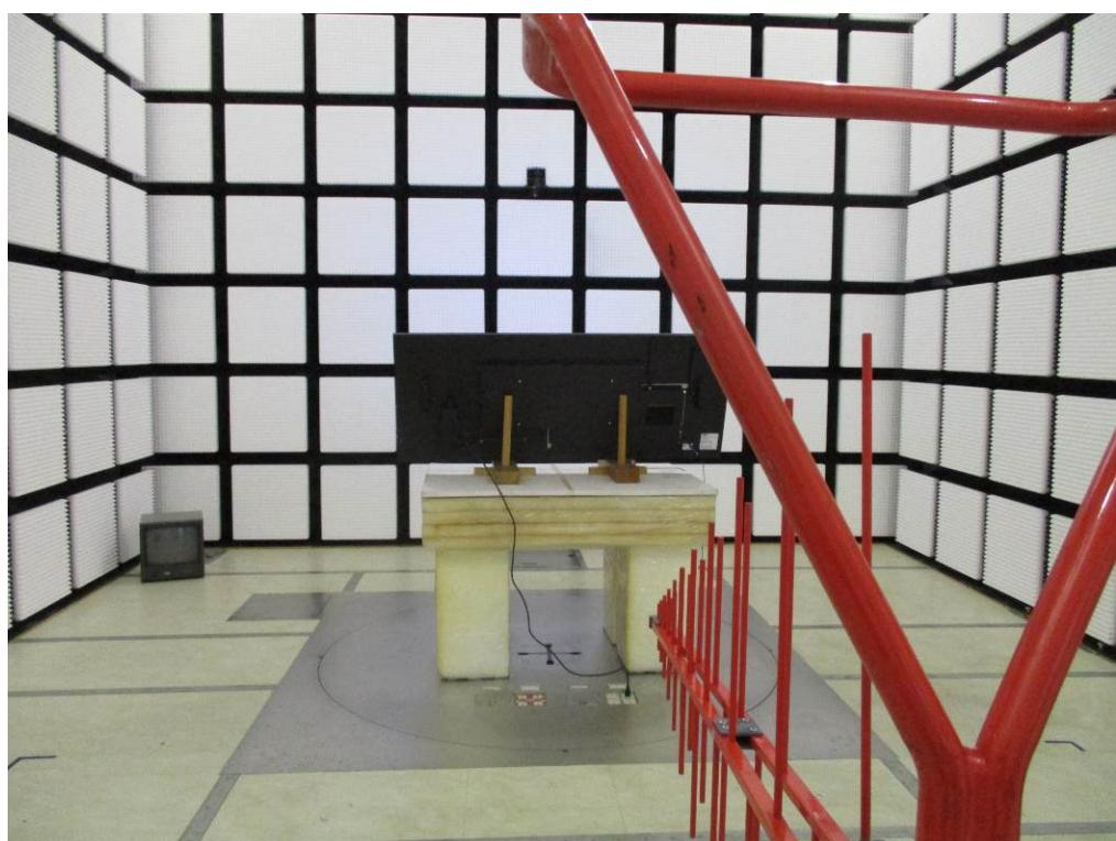
**RADIATED RF MEASUREMENT SETUP****Above 1 GHz**
