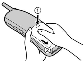
**2** Remove the old battery. Then install the new one.
