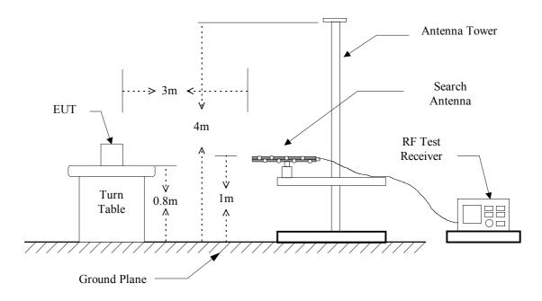
Figure 1: Frequencies measured below 1 GHz configuration
