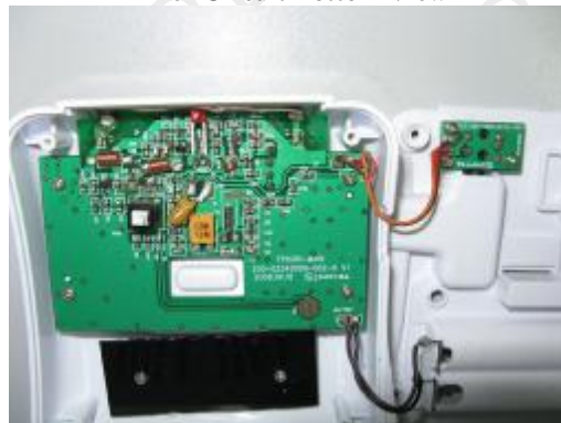
Inner Circuit Bottom View
