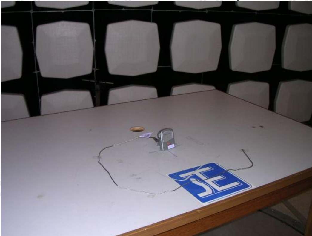
Measurement of Radiated Emission Test Set Up
