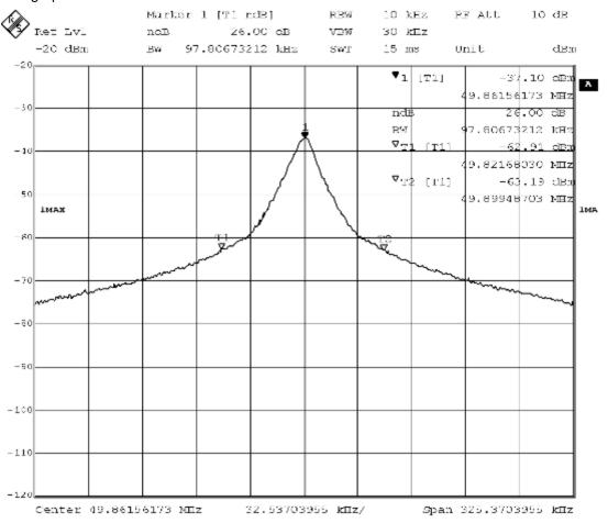
26dB bandwidth lower frequency :49.82168030MHz 26dB bandwidth upper frequency :49.89948703MHz
