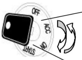
**Step 2:** Within a 10 second period after cycling the ignition for the 5<sup>th</sup> time, press button I. The car parking lights will flash once to confirm that the transmitter has been programmed. Continue program the additional remotes. The parking lights will flash two times when the programming mode is expired.
