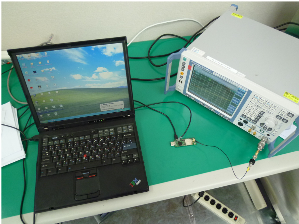
Photograph 4: Set-up for Conducted testing
