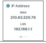
Function: Display WAN and LAN IP addresses (WAN IP address displays as 0.0.0.0 if not connected)
