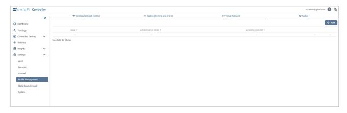
RADIUS (Remote Authentication Dial-In User Service) server profiles define external authentication servers used to validate wireless client credentials and control network access. Configuring RADIUS enables centralized authentication and policy management instead of using local credentials stored on each device.
