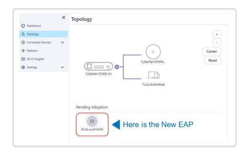
Step 3, Click the new EAP and then this EAP adds on the topology automatically.
