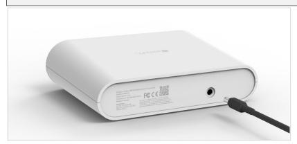
2. Using an Ethernet cable, connect your computer network port to the LAN port on the Controller. Refer to Figure 3.
