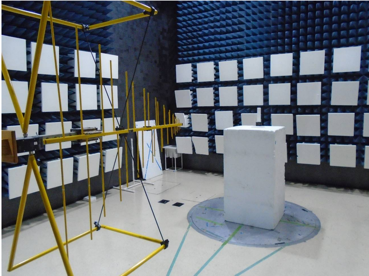
Figure 3: Typical Radiated Emissions – 30 MHz to 1 GHz shown
