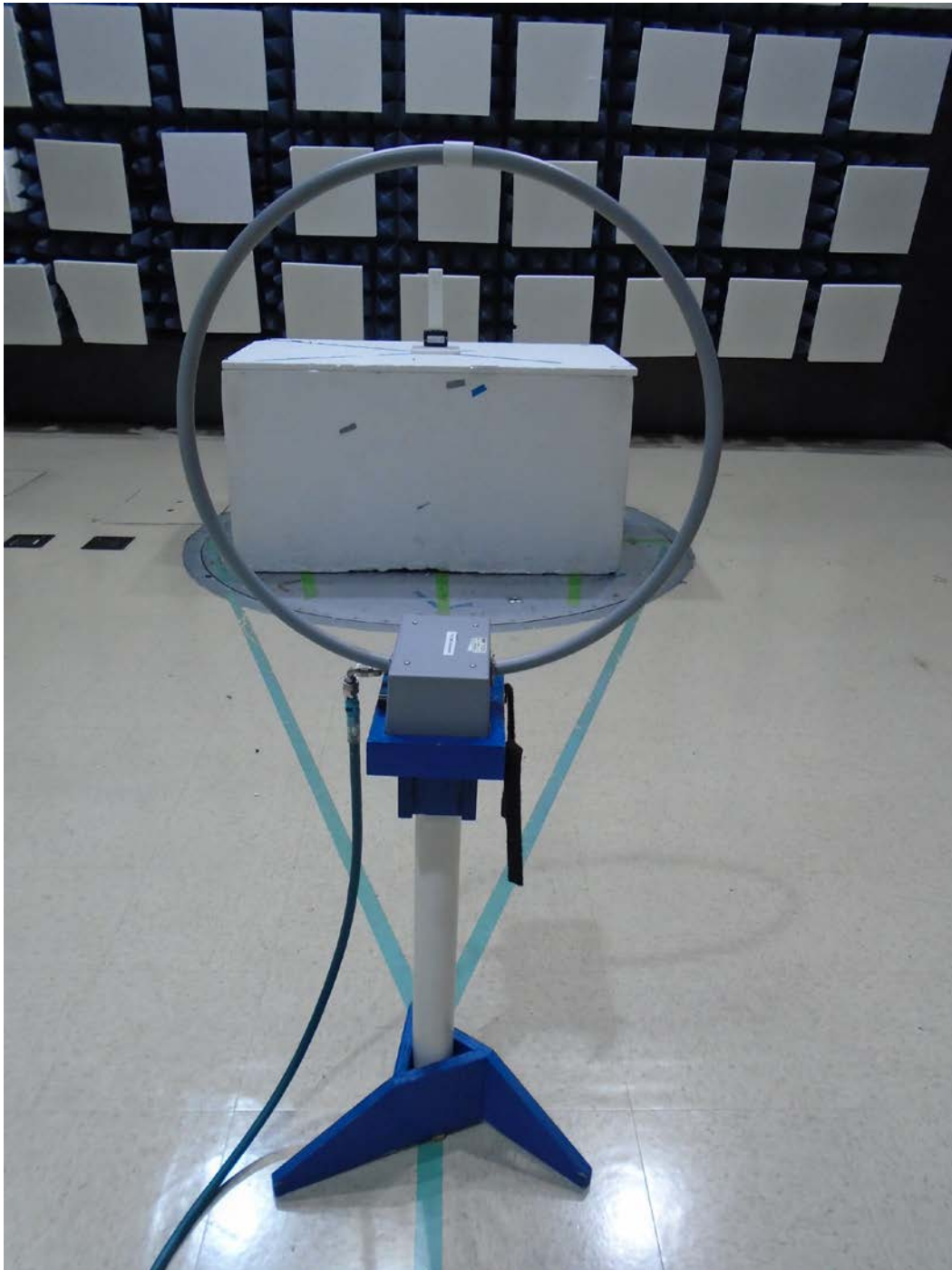
Figure 1: Typical Radiated Emissions – 10 kHz to 30 MHz shown, Parallel Orientation
