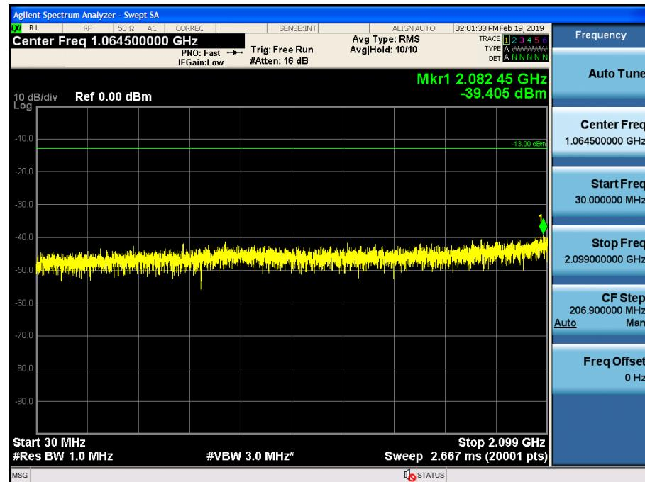
Spurious / AWS / Downlink / LTE 20 MHz / Middle / Low edge - 11 MHz ~ Low edge - 1 MHz
