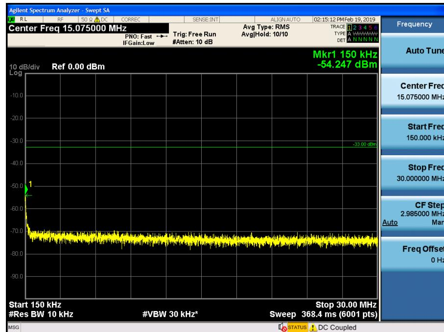
Spurious / AWS / Downlink / LTE 20 MHz / High / 30 MHz ~ Low edge - 11 MHz
