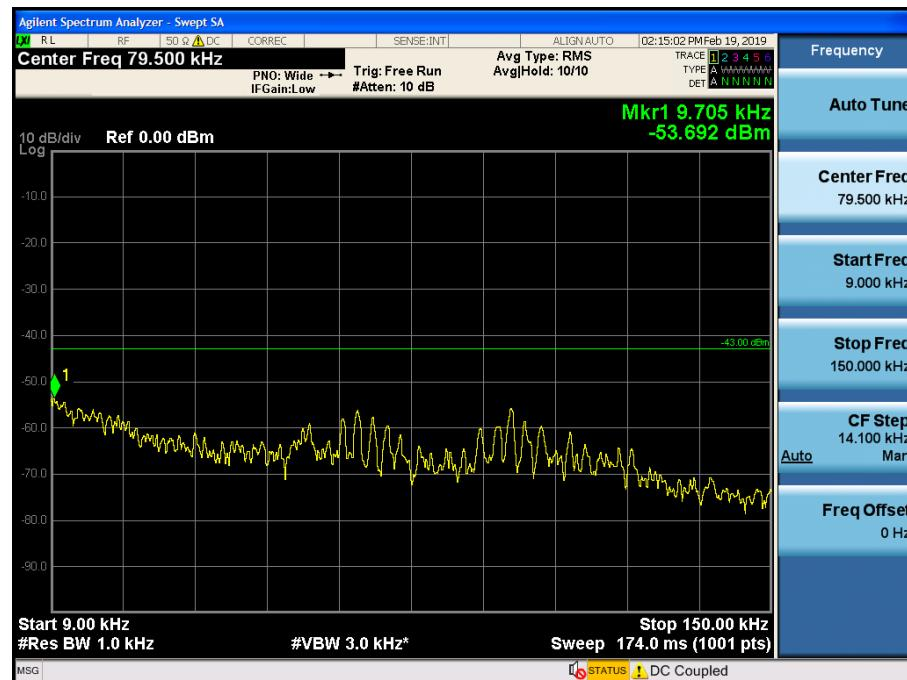
Spurious / AWS / Downlink / LTE 20 MHz / High / 150 kHz ~ 30 MHz
