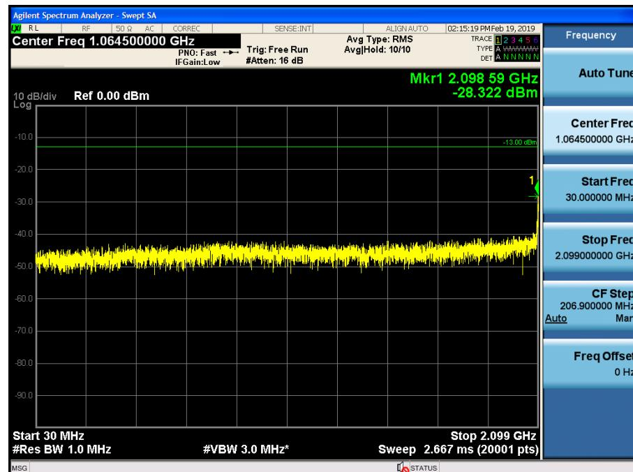
Spurious / AWS / Downlink / LTE 20 MHz / High / Low edge - 11 MHz ~ Low edge - 1 MHz
