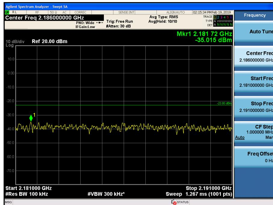
Spurious / AWS / Downlink / LTE 20 MHz / High / High Edge + 11 MHz ~ 10 GHz
