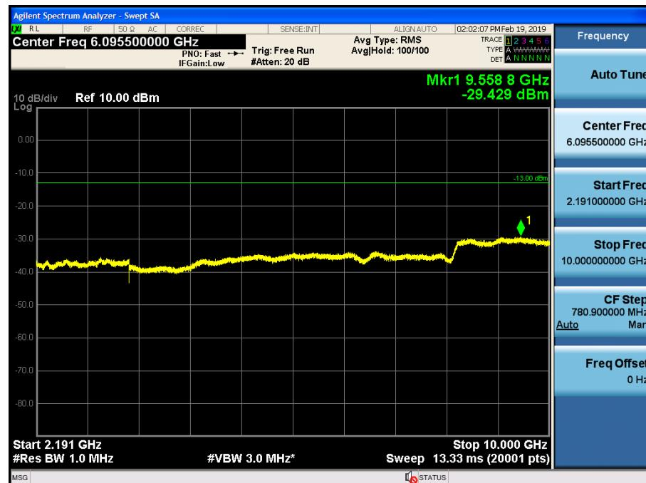
Spurious / AWS / Downlink / LTE 20 MHz / Middle / 10 GHz ~ 26.5 GHz
