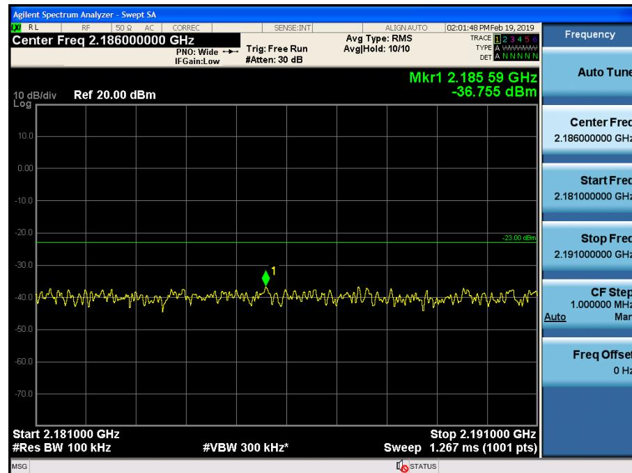
Spurious / AWS / Downlink / LTE 20 MHz / Middle / High Edge + 11 MHz ~ 10 GHz
