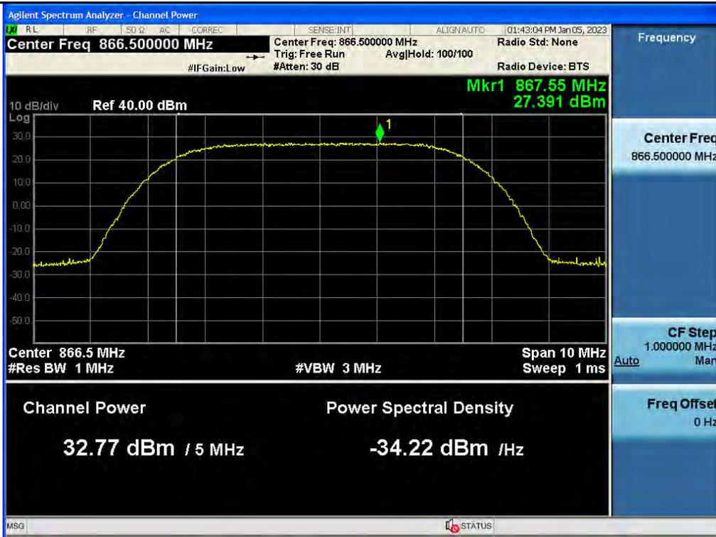
3 dB above the AGC threshold PSD / ESMR / Downlink / 5G NR 5 MHz
