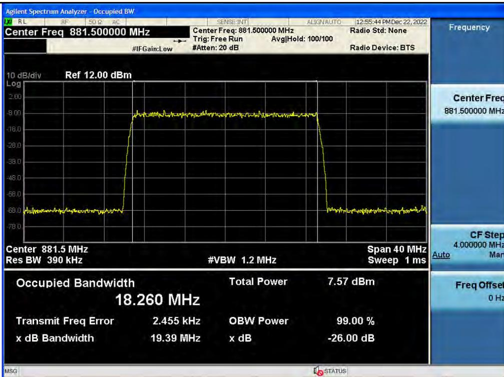
3 dB above the AGC threshold output / Cellular / Downlink / 5G NR 20 MHz
