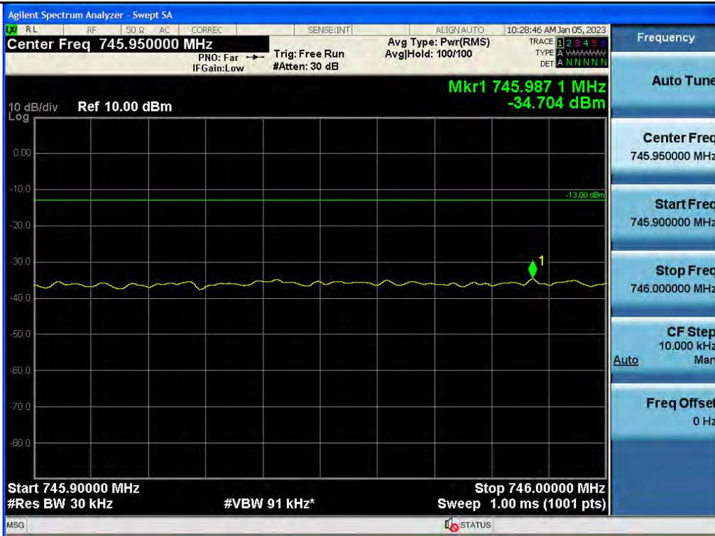
Out-of-band (single test signal) / Upper 700 MHz / Downlink / 5G NR 10 MHz / Upper
