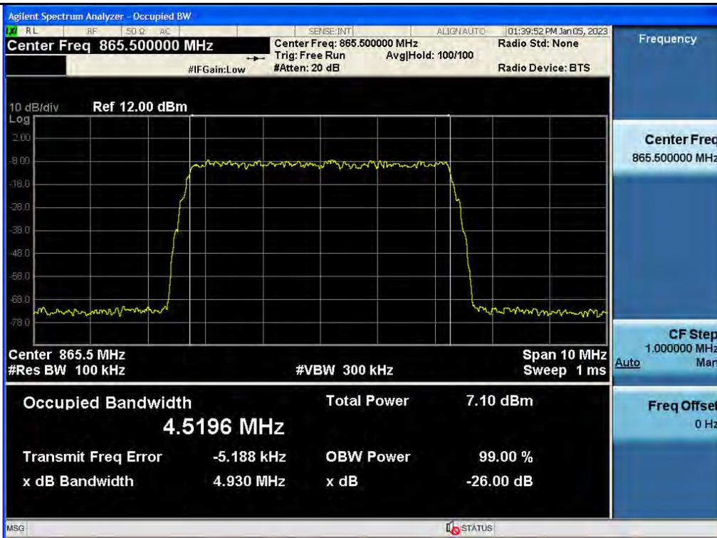
3 dB above the AGC threshold output / ESMR / Downlink / 5G NR 5 MHz
