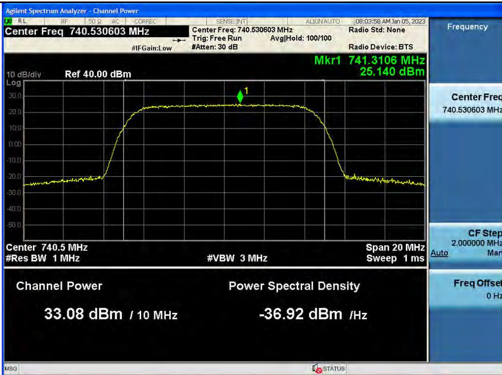
PSD / Upper 700 MHz / Downlink / LTE 10 MHz
