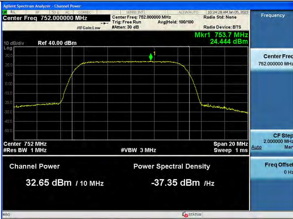
3 dB above the AGC threshold PSD / Upper 700 MHz / Downlink / 5G NR 10 MHz
