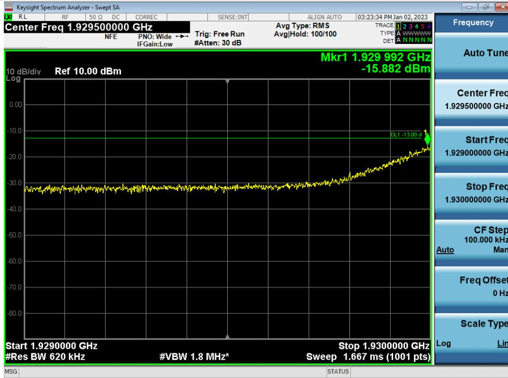
+3 dB above Out-of-band (single test signal) / PCS / Downlink / 5G NR 60 MHz / Upper
