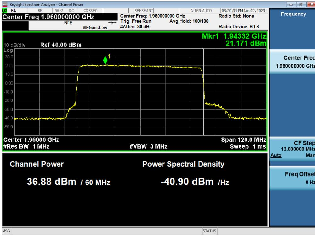
3 dB above the AGC threshold PSD / PCS / Downlink / 5G NR 60 MHz
