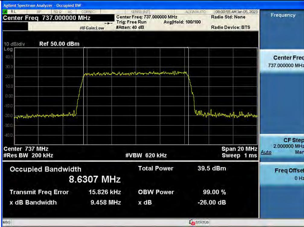
3 dB above the AGC threshold Input / Lower 700 MHz / Downlink / 5G NR 10 MHz
