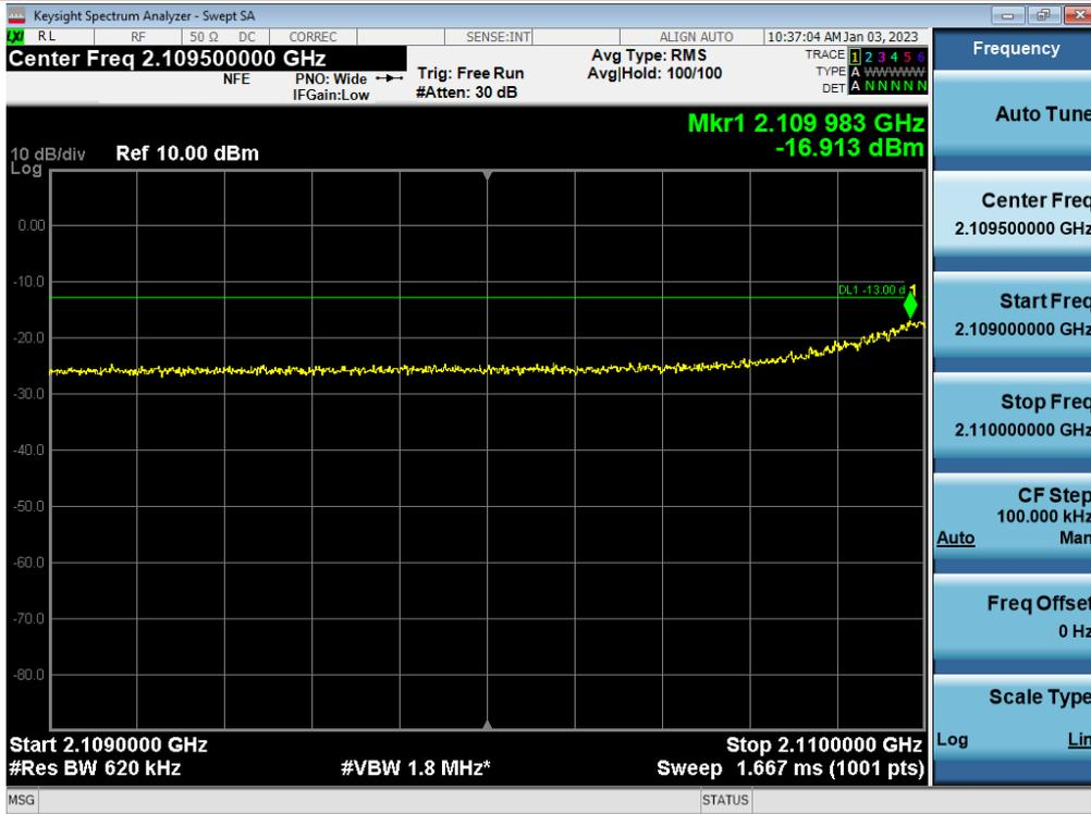
+3 dB above Out-of-band (single test signal) / AWS / Downlink / 5G NR 60 MHz / Upper
