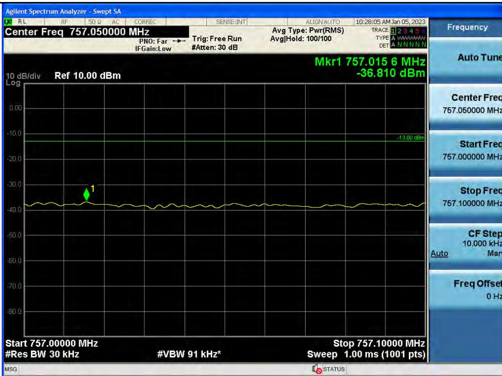
+3 dB above Out-of-band (single test signal) / Upper 700 MHz / Downlink / 5G NR 10 MHz / Lower
