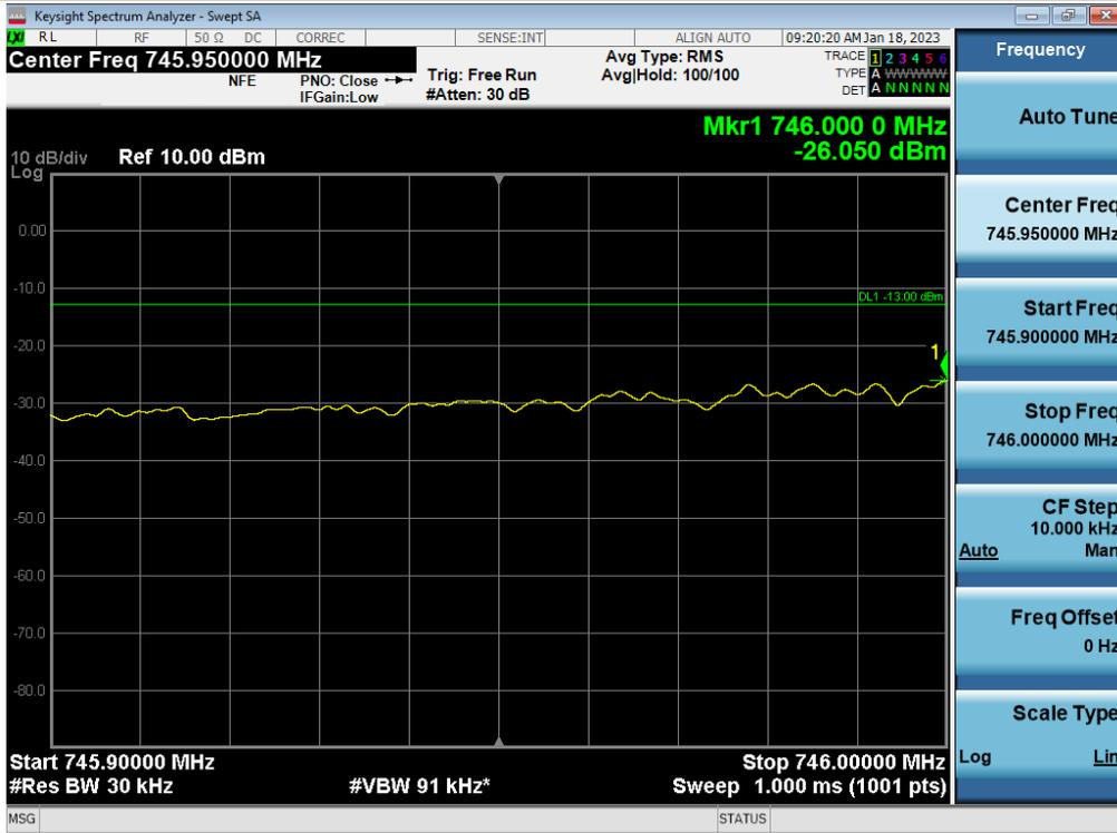
+3 dB above Out-of-band (single test signal) / Upper 700 MHz / Downlink / LTE 10 MHz / Upper
