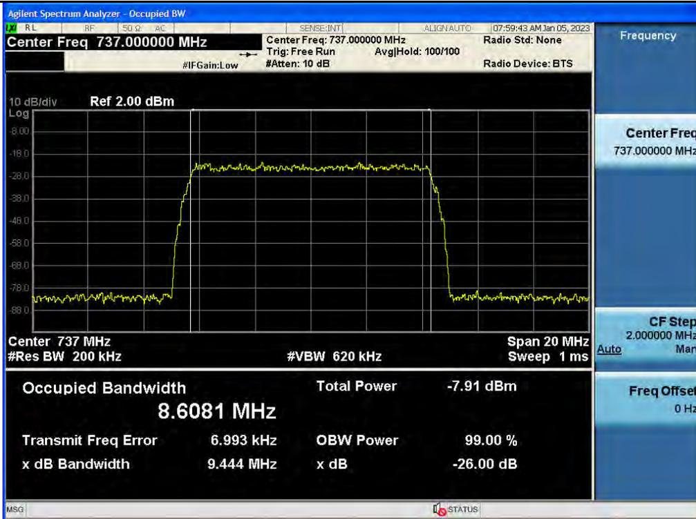
3 dB above the AGC threshold output / Lower 700 MHz / Downlink / 5G NR 10 MHz
