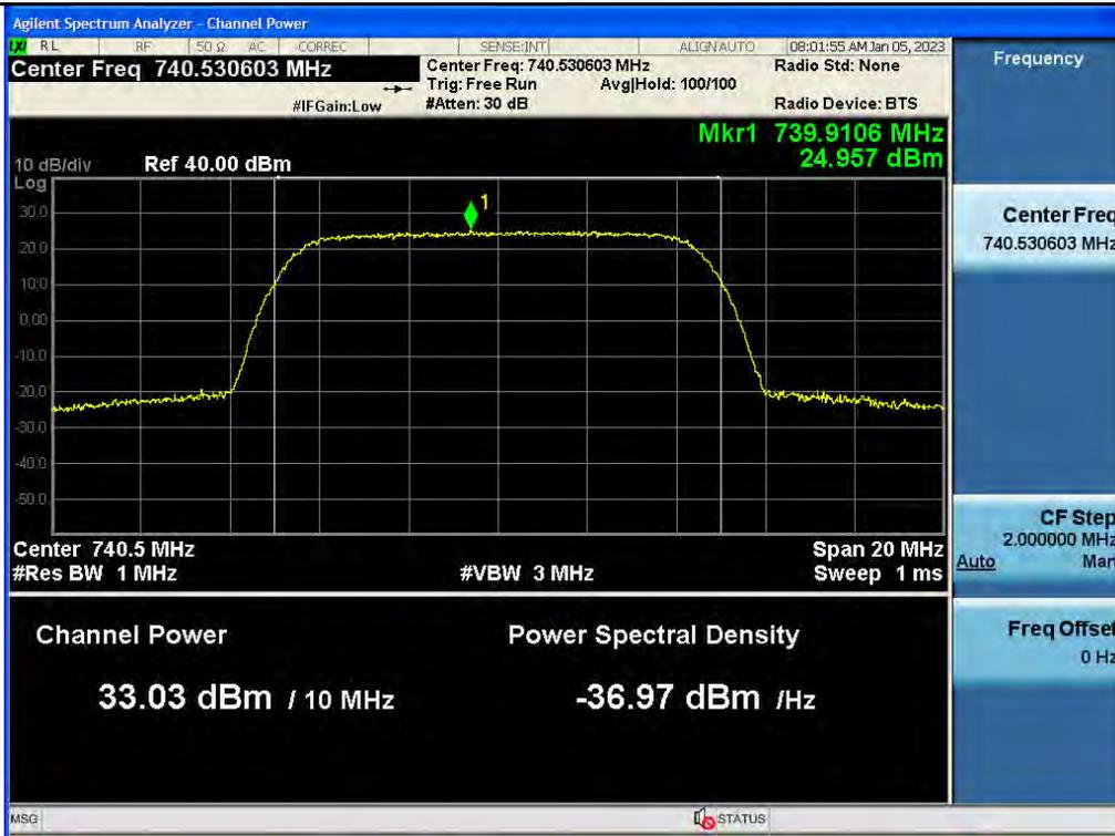
3 dB above the AGC threshold PSD / Lower 700 MHz / Downlink / 5G NR 10 MHz
