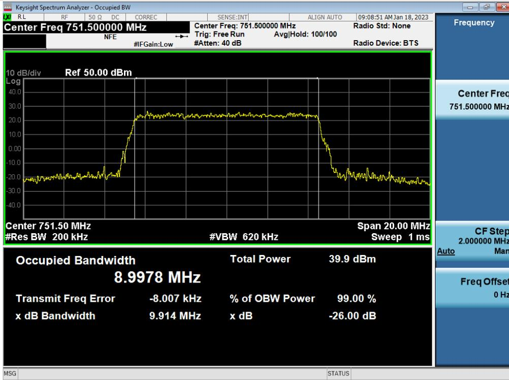
3 dB above the AGC threshold Input / Upper 700 MHz / Downlink / LTE 10 MHz
