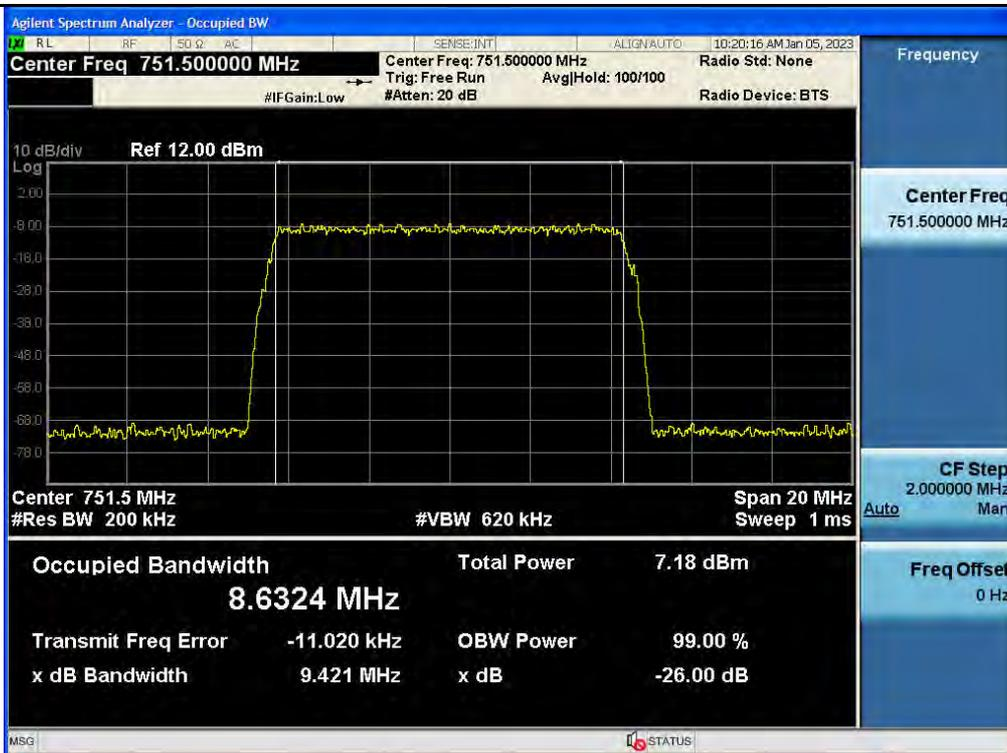
3 dB above the AGC threshold output / Upper 700 MHz / Downlink / 5G NR 10 MHz
