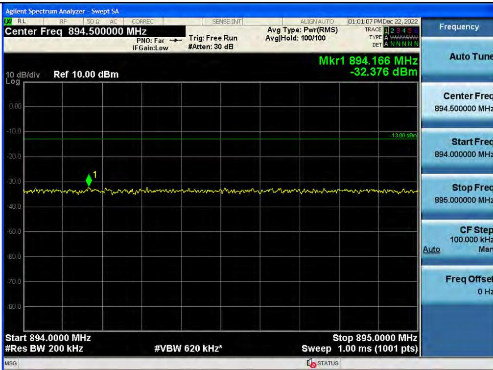
Out-of-band (single test signal) / AWS / Downlink / 5G NR 60 MHz / Lower
