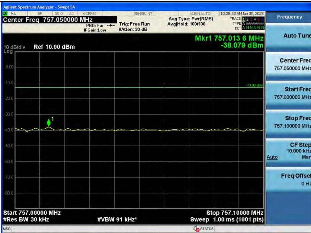
Out-of-band (single test signal) / ESMR / Downlink / 5G NR 5 MHz / Lower
