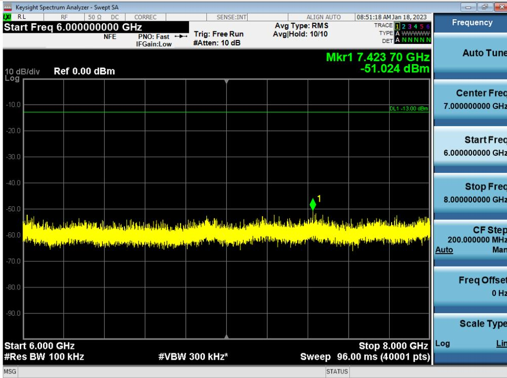
Spurious / Lower 700 MHz / Downlink / 5G NR 10 MHz / High / 9 kHz ~ 150 kHz
