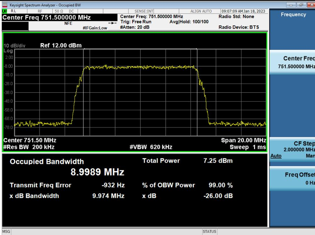
3 dB above the AGC threshold output / Upper 700 MHz / Downlink / LTE 10 MHz
