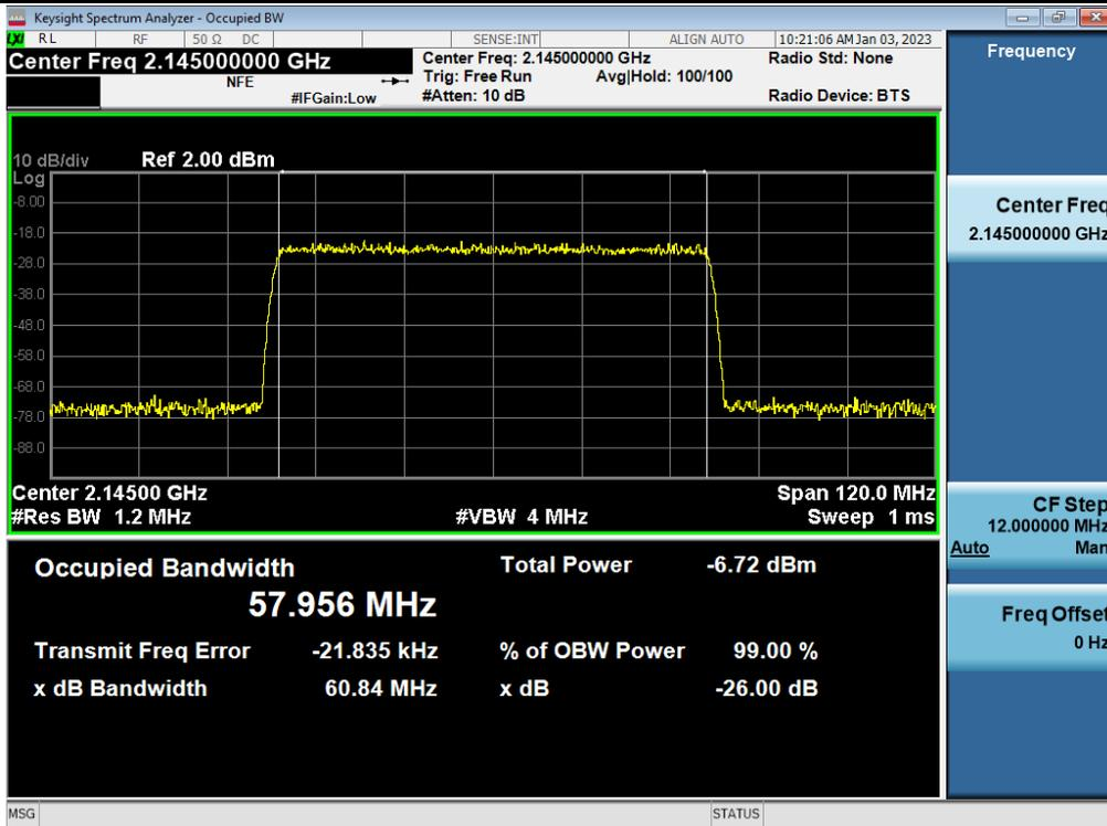
3 dB above the AGC threshold output / AWS / Downlink / 5G NR 60 MHz
