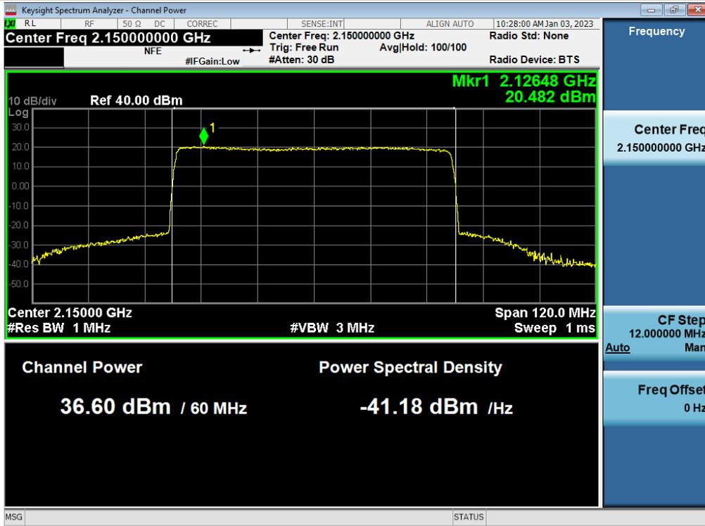
3 dB above the AGC threshold PSD / AWS / Downlink / 5G NR 60 MHz
