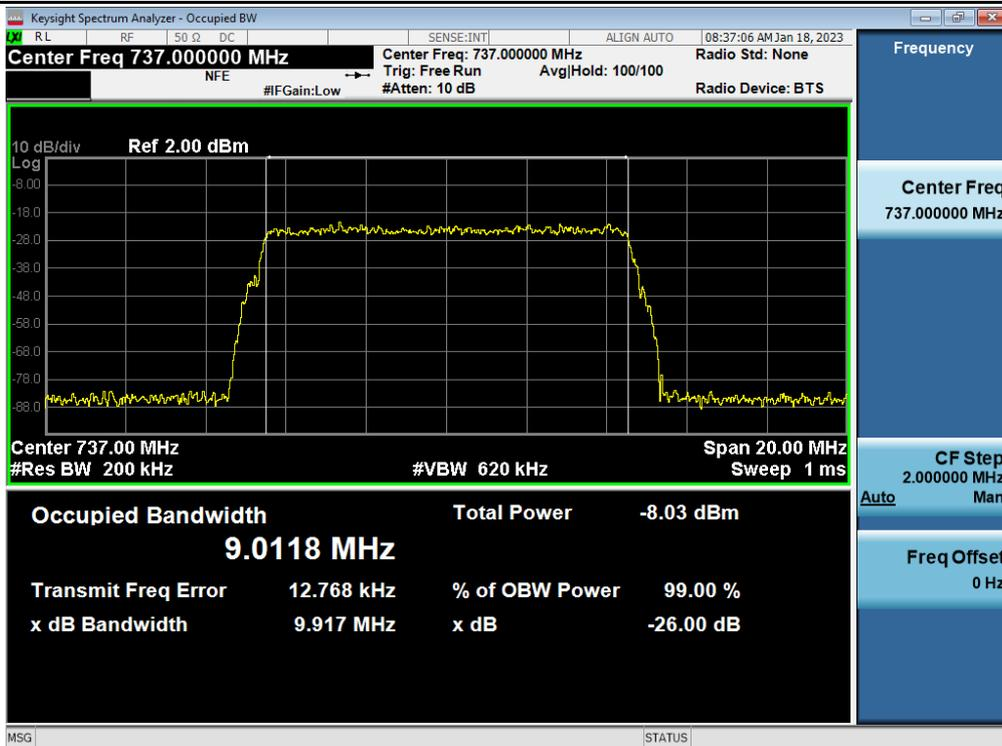
3 dB above the AGC threshold output / Lower 700 MHz / Downlink / LTE 10 MHz
