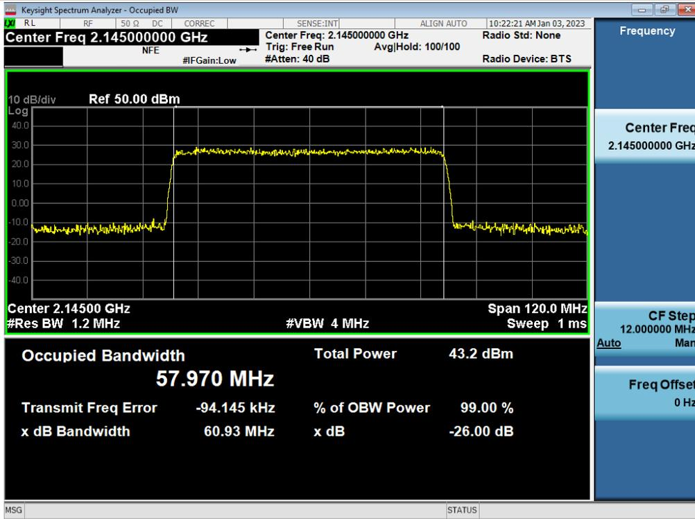
3 dB above the AGC threshold Input / AWS / Downlink / 5G NR 60 MHz
