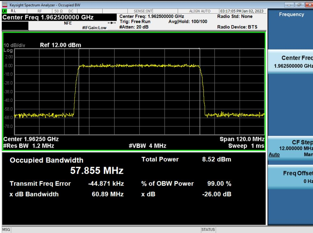
3 dB above the AGC threshold output / PCS / Downlink / 5G NR 60 MHz
