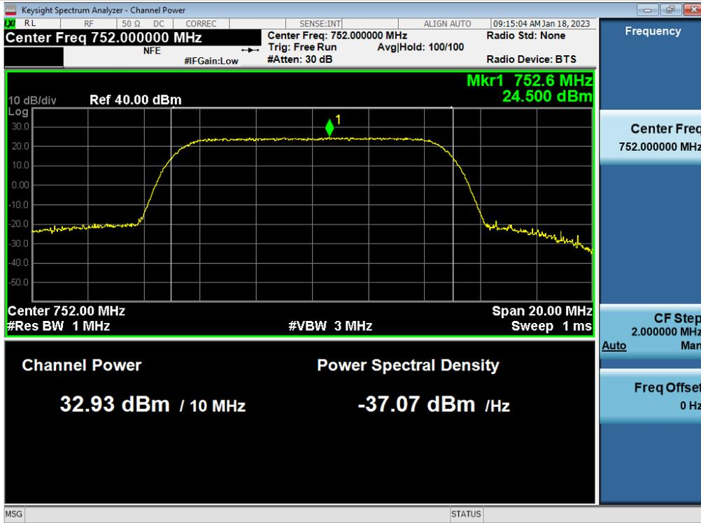
3 dB above the AGC threshold PSD / Upper 700 MHz / Downlink / LTE 10 MHz
