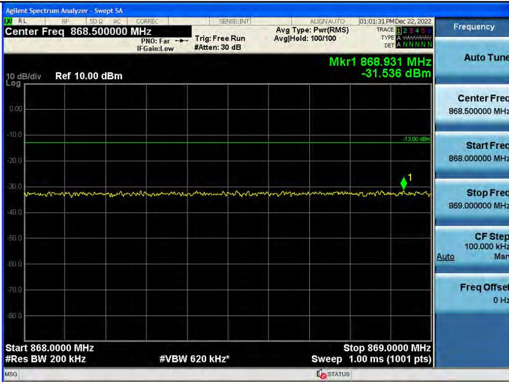
Out-of-band (single test signal) / Cellular / Downlink / 5G NR 20 MHz / Upper
