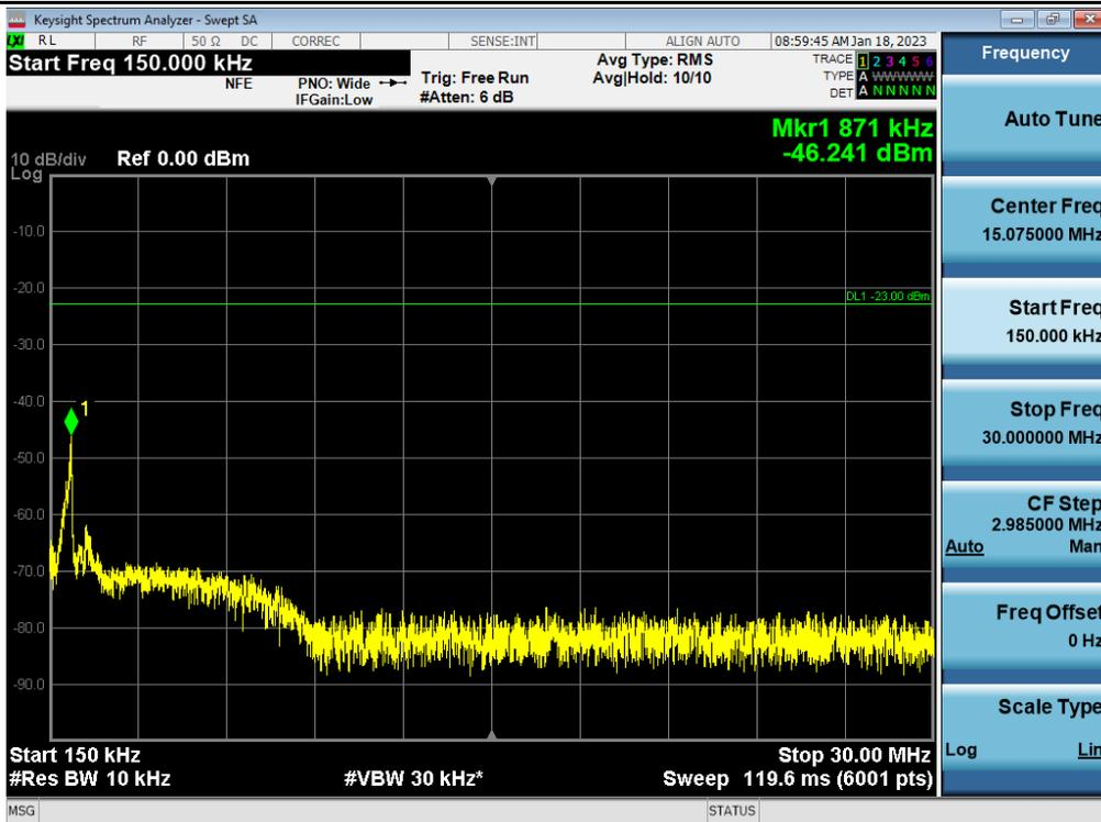
Spurious / Lower 700 MHz / Downlink / LTE 10 MHz / Middle / 30 MHz ~ Low Edge - 10 MHz
