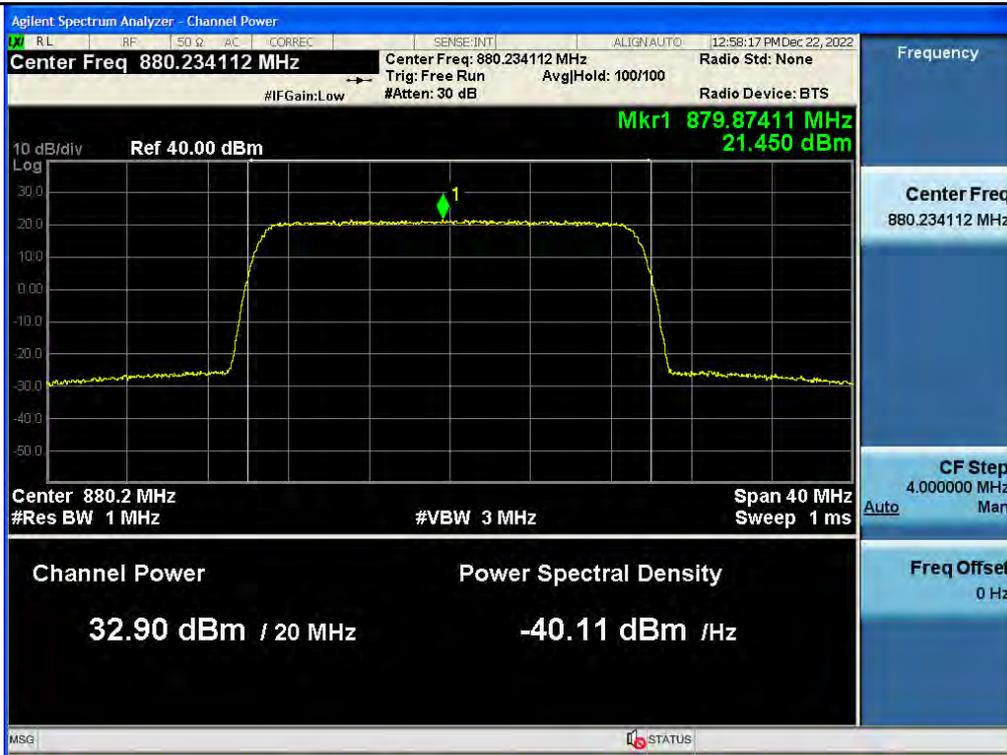
3 dB above the AGC threshold PSD / Cellular / Downlink / 5G NR 20 MHz
