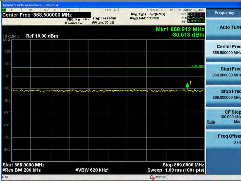
+3 dB above Out-of-band (single test signal) / Cellular / Downlink / 5G NR 20 MHz / Upper
