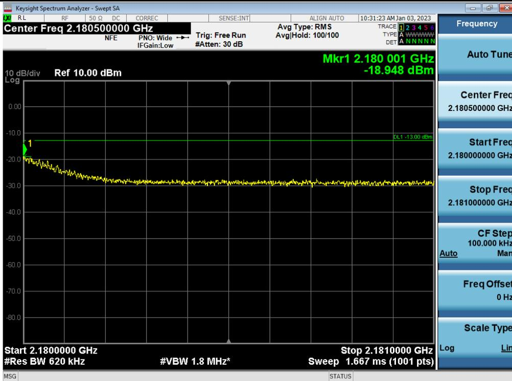
Out-of-band (single test signal) / PCS / Downlink / 5G NR 60 MHz / Lower
