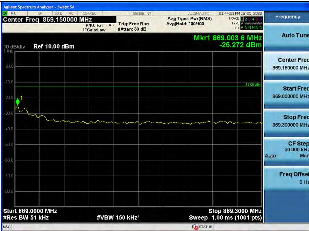
+3 dB above Out-of-band (single test signal) / ESMR / Downlink / 5G NR 5 MHz / Lower
