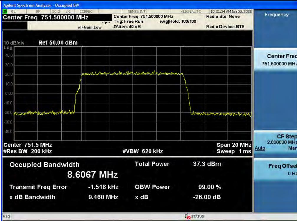
3 dB above the AGC threshold Input / Upper 700 MHz / Downlink / 5G NR 10 MHz
