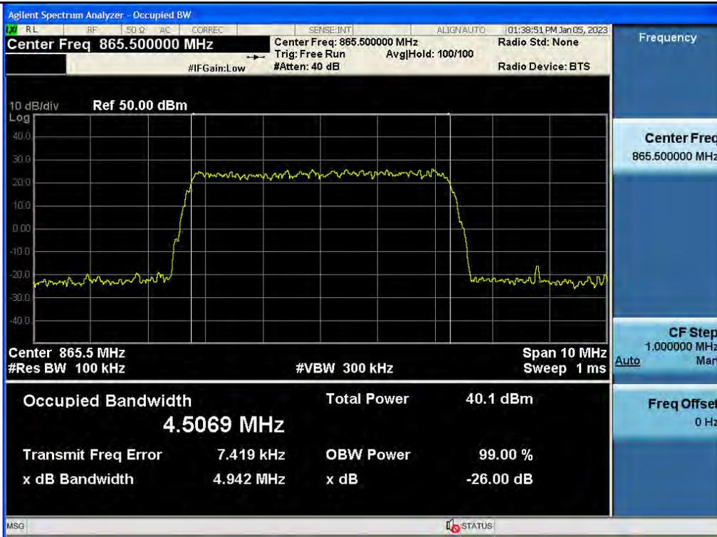
3 dB above the AGC threshold Input / ESMR / Downlink / 5G NR 5 MHz
