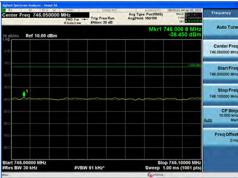
Out-of-band (single test signal) / Upper 700 MHz / Downlink / LTE 10 MHz / Lower
