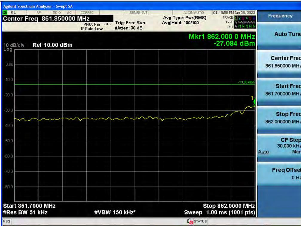
+3 dB above Out-of-band (single test signal) / ESMR / Downlink / 5G NR 5 MHz / Upper
