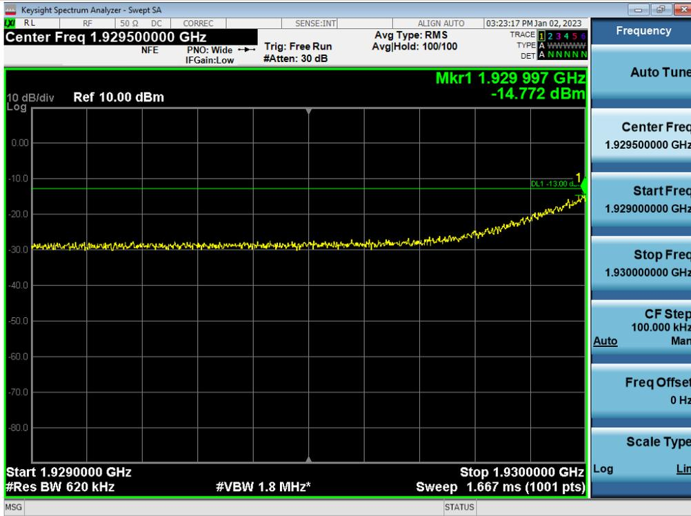
Out-of-band (single test signal) / PCS / Downlink / 5G NR 60 MHz / Upper
