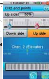
CH2摇杆打到最右边 CH2 stick to the far right (Pic 21.2)
