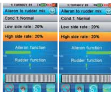
副翼摇杆打到最左边 Aileron to the far left (Pic 21.6)
