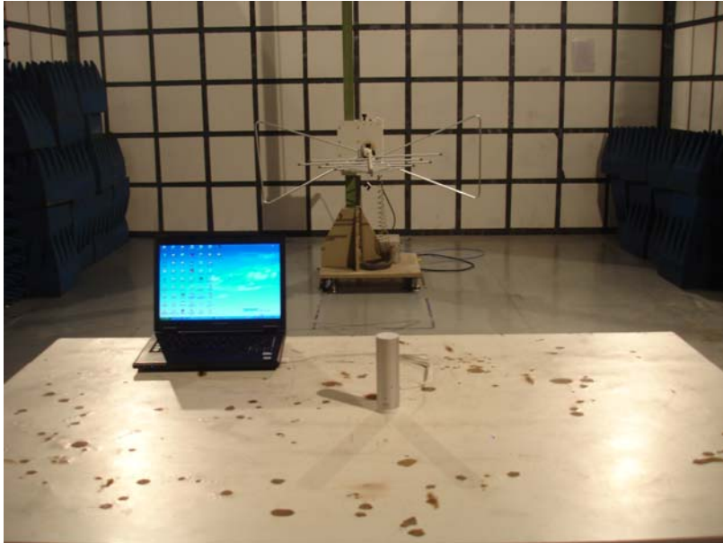
Photo of Setup for Radiated Emission (Indoor) (Below 1 GHz)
