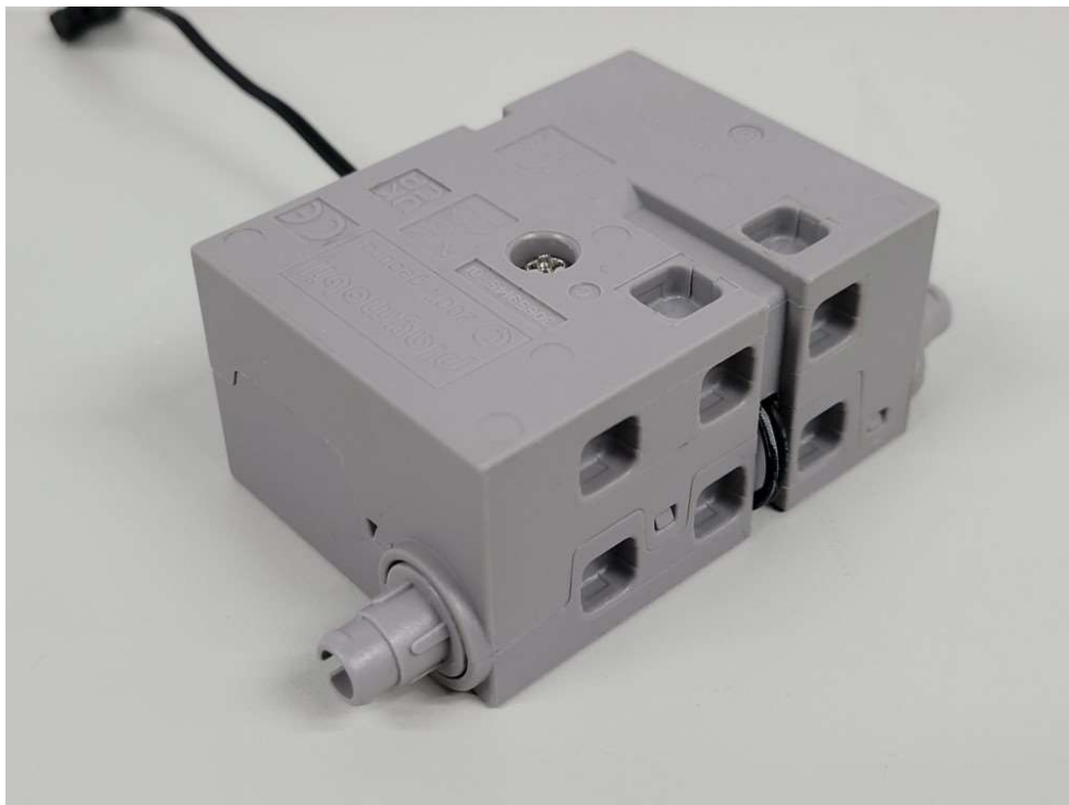
External View – Gear Box
