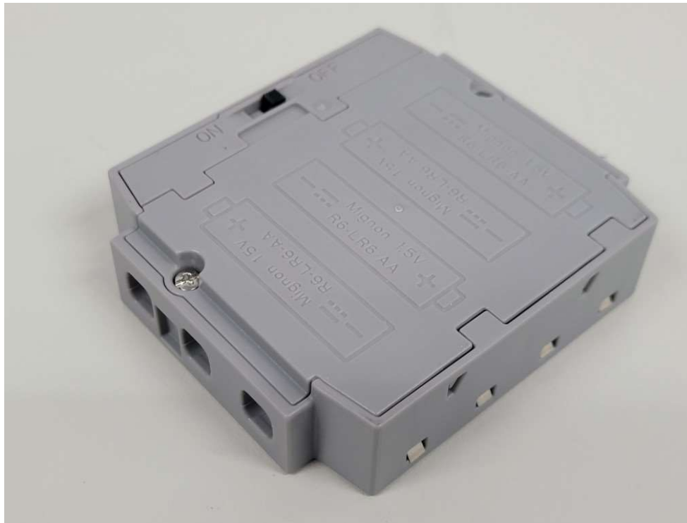
External View – Battery Box
