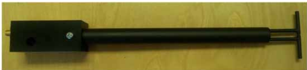
Figure 1 – MVG COMOSAR Validation Dipole
