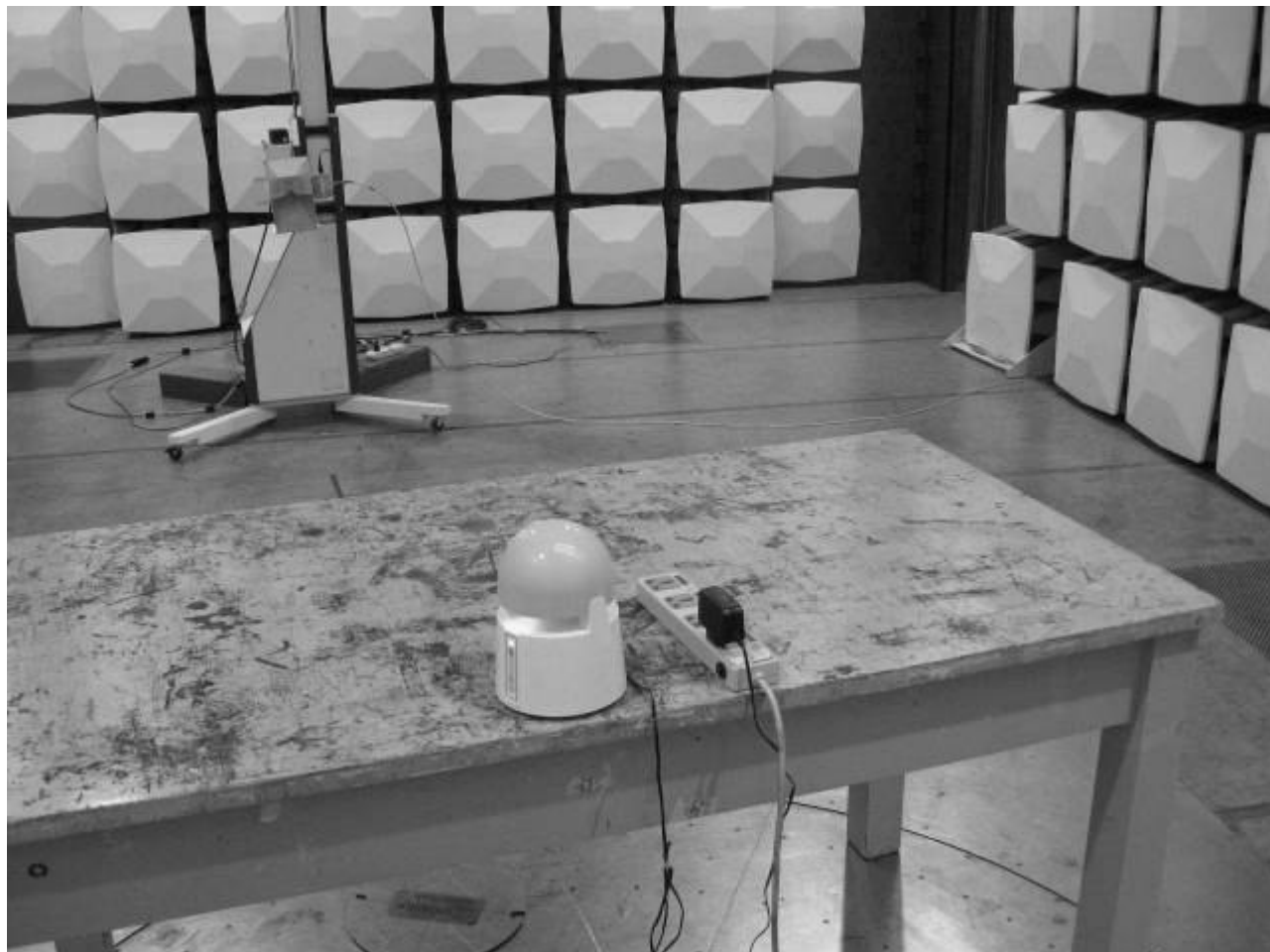
Photograph 3: Set-up for Radiation Measurement above 1GHz
