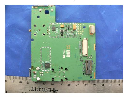
**EUT – Radio Board side 2 view 1 (with shielding)**
