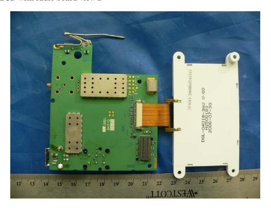
**EUT – Radio Board side 1 view 1 (with shielding)**
