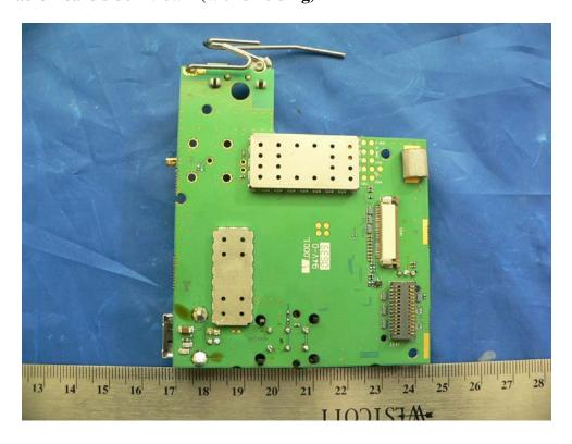
**EUT – Radio Board side 1 view 2 (without shielding)**
