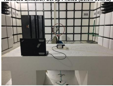
Radiated Emission Set up Photos (Below 1GHz)
