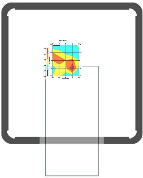
1 gram SAR value : 0.126 W/kg 10 gram SAR value : 0.062 W/kg Area Scan Peak SAR : 0.150 W/kg Zoom Scan Peak SAR: 0.226 W/kg
