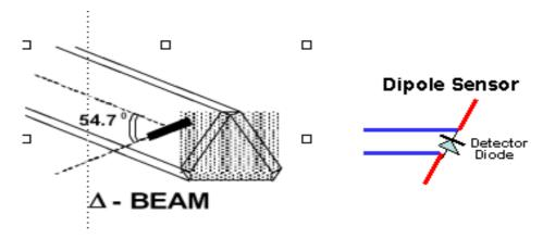
SAR is assessed with a calibrated probe which moves at a default height of 5mm from the center of the diode, which is mounted to the sensor, to the phantom surface (in the Z Axis). The 5mm offset height has been selected so as to minimize any resultant boundary effect due to the probe being in close proximity to the phantom surface.
