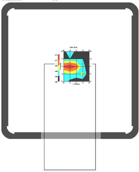
1 gram SAR value : 0.126 W/kg 10 gram SAR value : 0.071 W/kg Area Scan Peak SAR : 0.150 W/kg Zoom Scan Peak SAR: 0.244 W/kg
