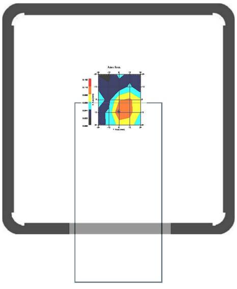
1 gram SAR value : 0.135 W/kg 10 gram SAR value : 0.074 W/kg Area Scan Peak SAR : 0.162 W/kg Zoom Scan Peak SAR: 0.331 W/kg
