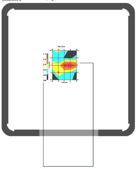
1 gram SAR value : 0.149 W/kg 10 gram SAR value : 0.071 W/kg Area Scan Peak SAR: 0.175 W/kg Zoom Scan Peak SAR: 0.340 W/kg
