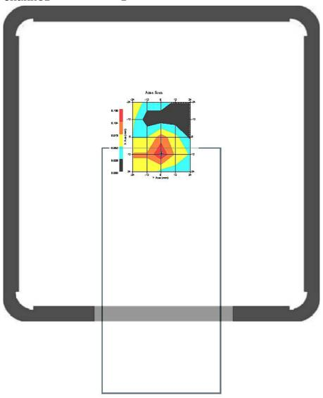
1 gram SAR value : 0.124 W/kg 10 gram SAR value : 0.063 W/kg Area Scan Peak SAR : 0.140 W/kg Zoom Scan Peak SAR: 0.241 W/kg
