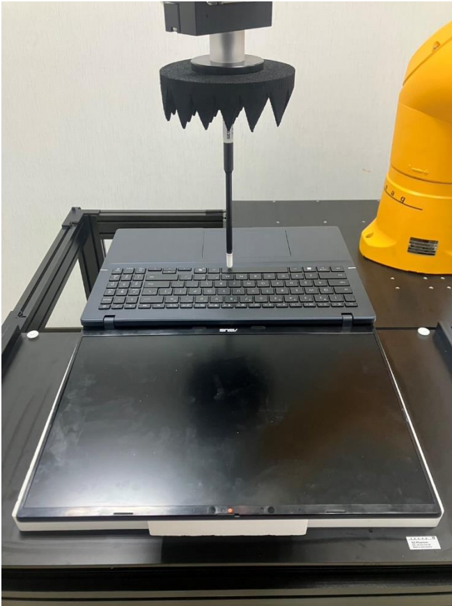
Testing Setup for Power Density, Top Side of KeyBoard at 2 mm
