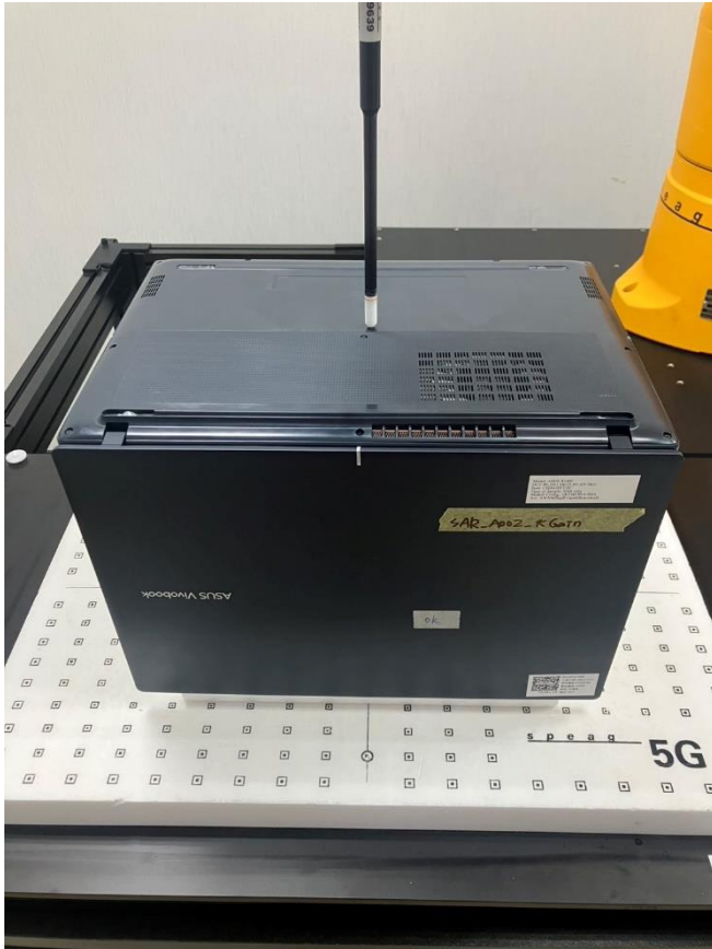
Testing Setup for Power Density, Bottom of Laptop at 2 mm
