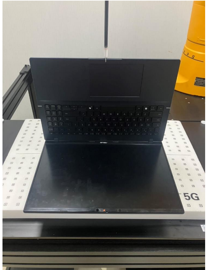
Testing Setup for Power Density, Front Edge of laptop at 2 mm
