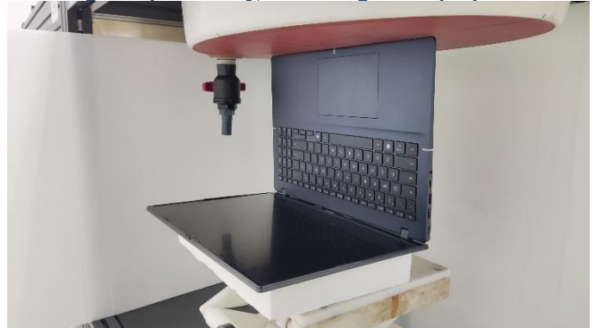
Testing Setup for Body, Front Edge of Laptop at 0 mm
