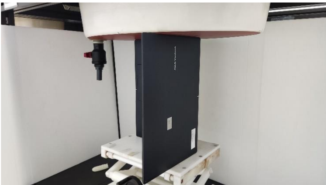
Testing Setup for Extremity, Left Edge of laptop at 0 mm
