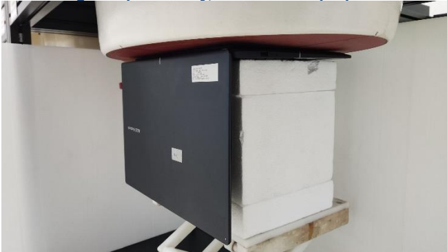
Testing Setup for Body, Bottom of Laptop at 0 mm
