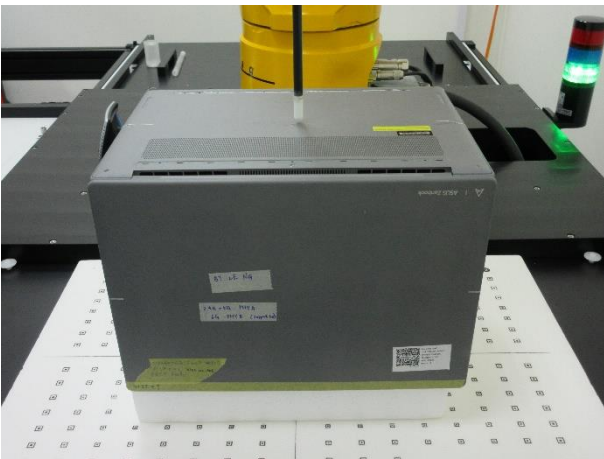
Testing Setup for Power Density, Bottom of Laptop at 2 mm
