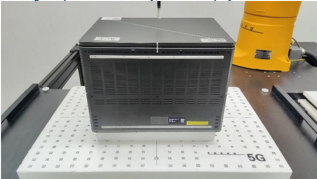
Testing Setup for Power Density, Back of Display Screen at 25 mm
