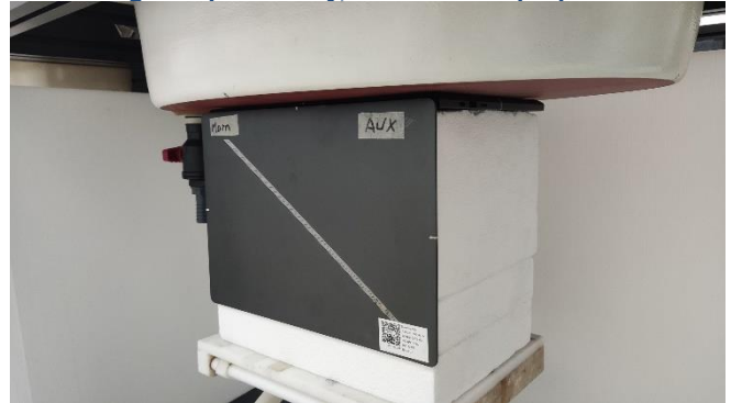
Testing Setup for Body, Bottom of Laptop at 0 mm
