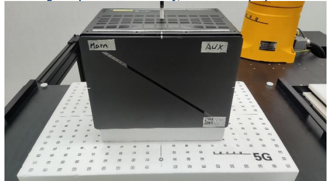
Testing Setup for Power Density, Bottom of Laptop at 2 mm
