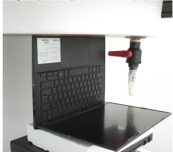
Testing Setup for Body, Front Side of Laptop at 0 mm
