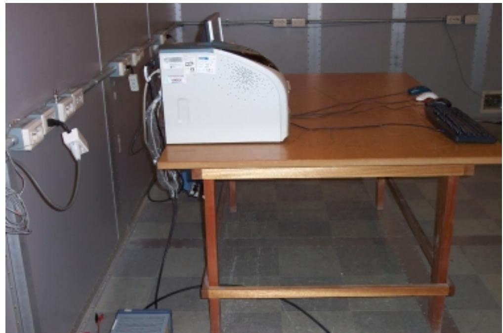
● **Radiated Test Picture(Front)**
