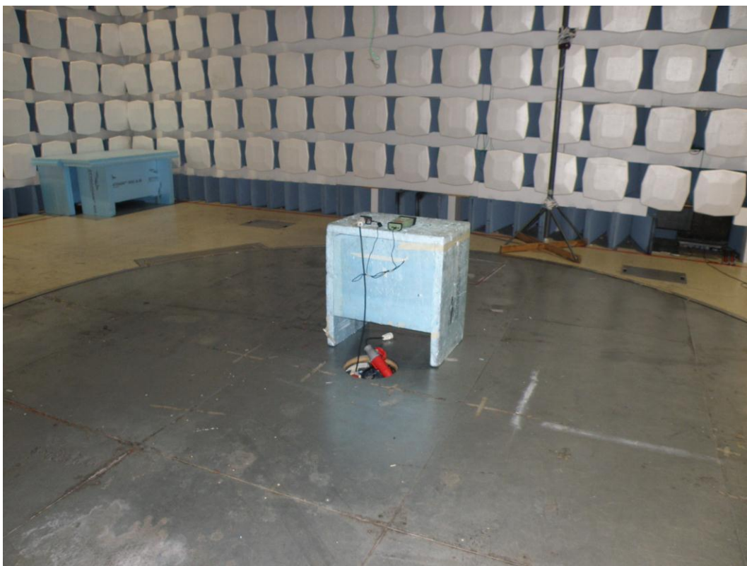
Photograph 1. Radiated spurious emission test.
