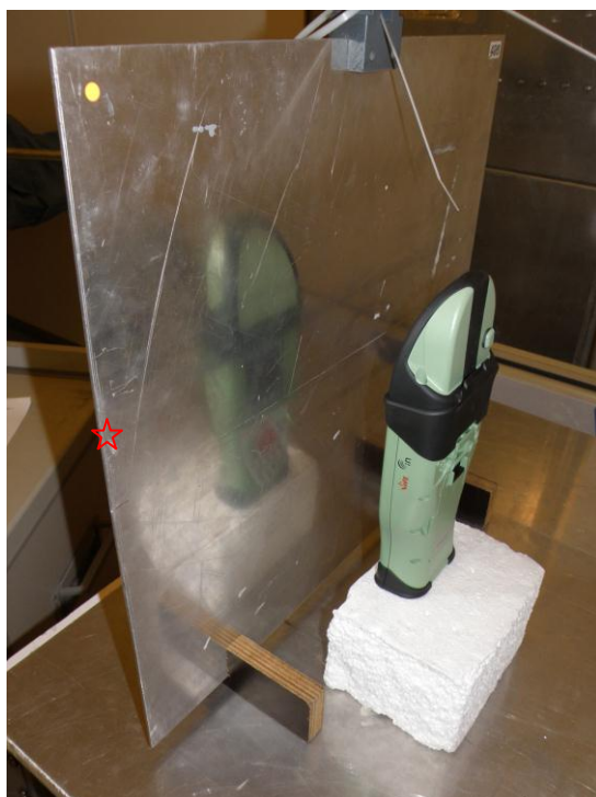
Photograph 4. Electrostatic discharge (ESD) immunity test.
