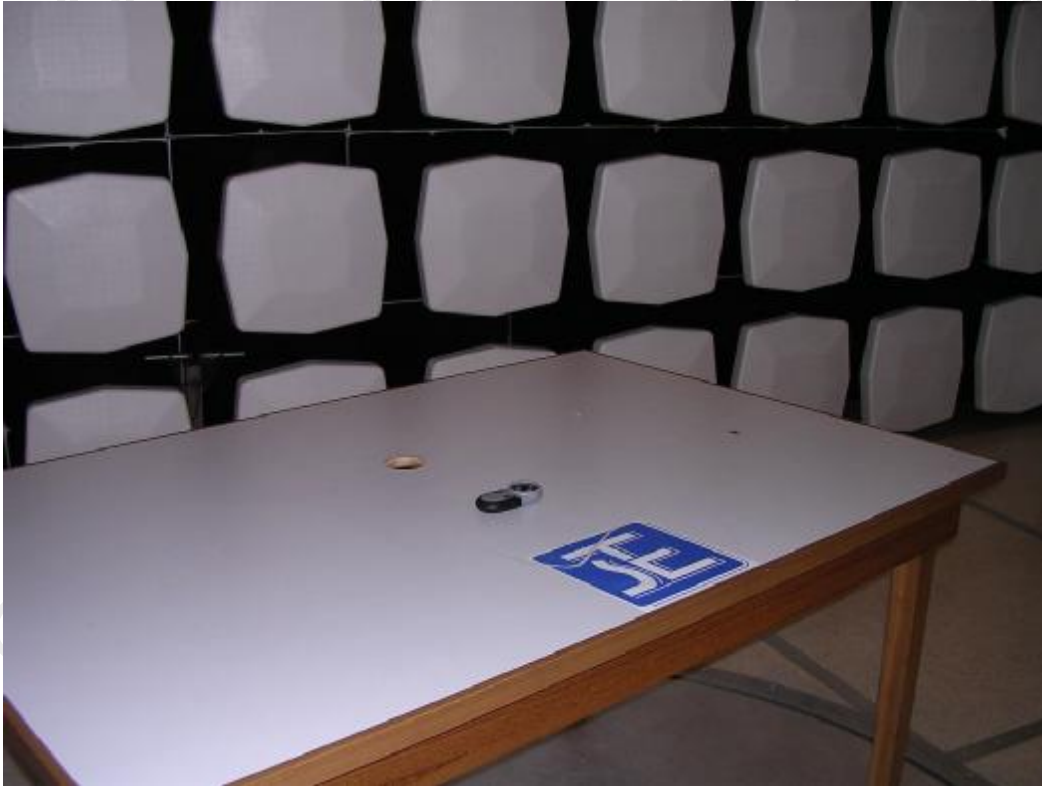
Measurement of Radiated Emission Test Set Up
